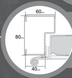
Zinc coated, robust and maintenance free steel frame. Painted same colour as the door or different if specified.
