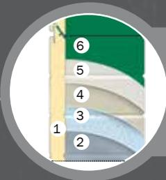
Energy efficient insulated door panels. Double steel skin filled with freon free PU foam: 1- 40mm thick foam; 2- steel; 3- zinc; 4- primer; 5- finish coating; 6- colour.
