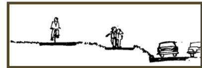
Figure 9.2.2 - Separate pedestrian/ bicycle/ vehicular access
