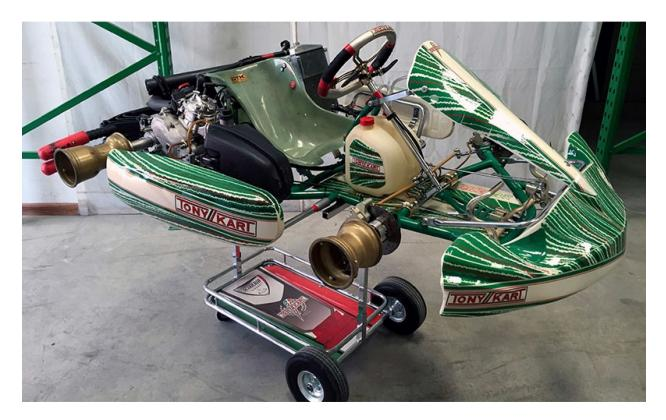
Few karting tools or pieces of equipment are as helpful as a kart stand. These stands make it easy to move the kart from your pit to the grid, and work on the kart with little hindrance. Many stands, like the one pictured, have a small tray for tools and parts, and can fold or collapse to be easier to transport. (PC: KartDubai)
