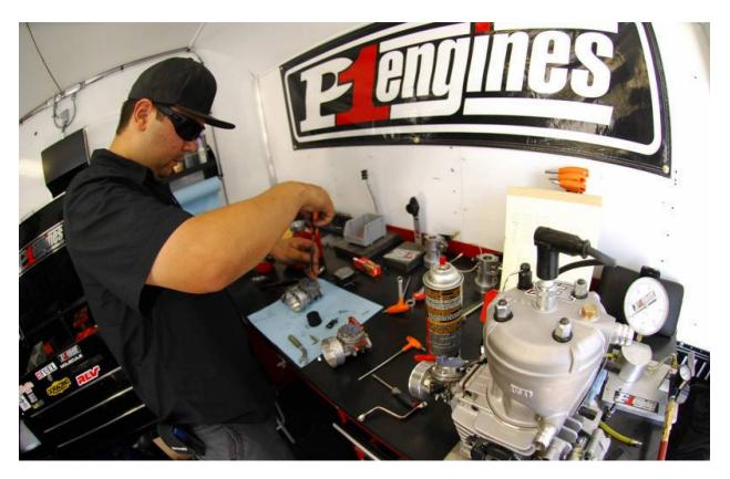
While you may not need one initially, many kart racers will utilize a motor builder or service technician to ensure that their engine package is within technical, wear, and service limits. Motor builders have the tools and knowledge to help you find the performance and reliability you need out of your kart engine. Here, a motor builder reassembles a carburetor after replacing some of the smaller gaskets and parts within it. (PC: OnTrack Promotions)
