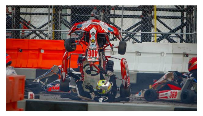
By design, karts do not usually have a roll cage or seat belts installed in them. In an accident such as this one, the driver is considered safer by falling out of the kart than remaining squarely in the seat, where the full weight of the kart could be placed upon his head and neck. In this accident, a driver's rib vest, helmet, and suit keep him safe from the kart and the abrasion of the track. (PC: OnTrack Promotions)
