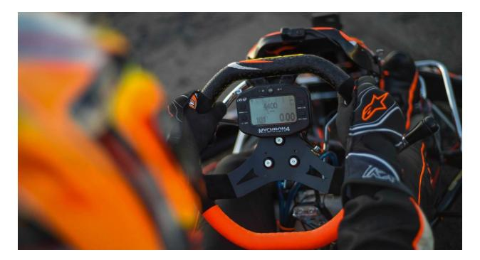
A data acquisition system like this one, pictured attached to a driver's steering wheel, is highly useful for many reasons. Depending on the functions the system has, a driver and kart's lap time, RPM, engine temperature, and even GPS position on the track can be found within the data these systems store or display in real time. (PC: OnTrack Promotions)
