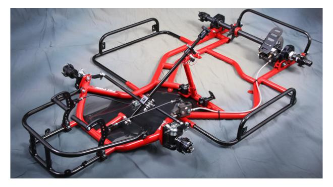
An oval track kart chassis, with seat, tires, and bodywork removed. Note the offset chassis structure (naturally to the left). In many ways, this chassis is exactly the same as a sprint kart chassis, but critical components like the driver's seat position, steering, and even bodywork are offset to cater to left turns.(PC: Southern Express Karting)
