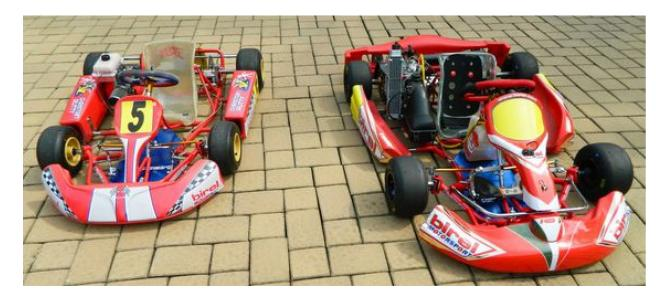
Drivers of different ages can enter into karting through the class system, which allows for a progressive increase in the size of the kart, and resultant performance. Here, a kid kart (left) sits alongside a cadet kart powered by a Rotax MicroMax engine. (PC: Radne)
