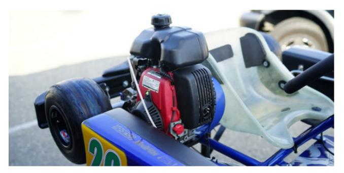
In recent years, the Honda Gxh50 engine has been the go-to engine package for most Kid Kart classes across the country. 50cc engines produce between 2 and 4 horsepower, and will propel a Kid Kart to a top speed of roughly 40 mph. (PC: Ekartingnews.com)
