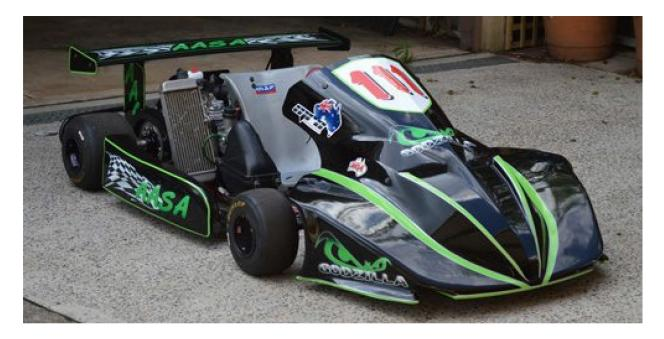
Another slight variation on road racing and endurance karts are so called 'super karts.' With large engines, tires, and often additional aerodynamic bodywork, these karts are capable of speeds at times in excess of 150 miles per hour. While not as common a sight at the track, they are hard to miss when they are there, as their pace through the corners and down the straightaways is dramatic. (PC: KartPulse)
