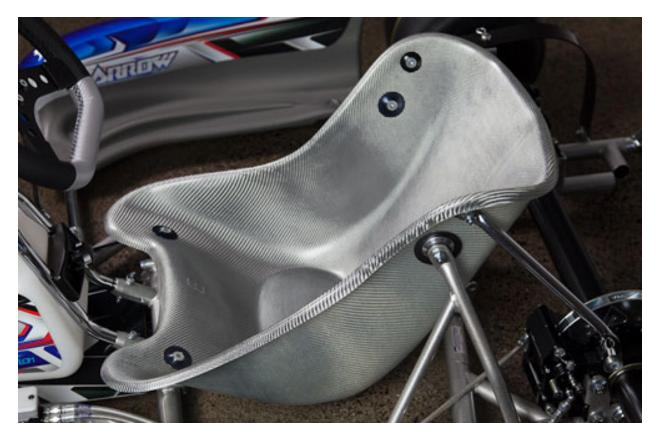
The kart seat has evolved over the years considerably. Note the flat bottom of this seat, which allows for a lower mounting position. The silver-sheen of this karting seat suggests that this seat features reinforced cross-weaving of the fiberglass, which ads durability and performance. Also, note the silver seat strut mounted to the rear of the seat, providing additional grip to the rear tires. (PC: KartSport NZ)
