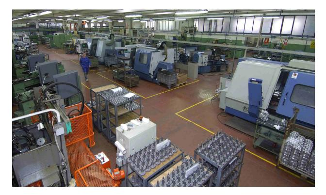
Kart engines of today are produced using advanced materials, manufacturing techniques, and computer-aided design to ensure that the greatest level of parity between each engine is achieved. In this photo, the CNC machines and manufacturing floor of an IAME Karting Engine factory is shown. (PC: IAME Karting)
