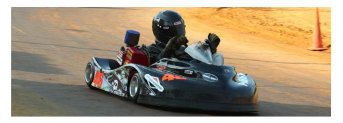
While 4-cycle engines are becoming more prevalent in all types of kart racing, the premier example of the potential of 4-cycle engine packages in karting has consistently been oval track karting events. Almost all oval karts are powered by 4-cycle engines. (PC: TKA)
