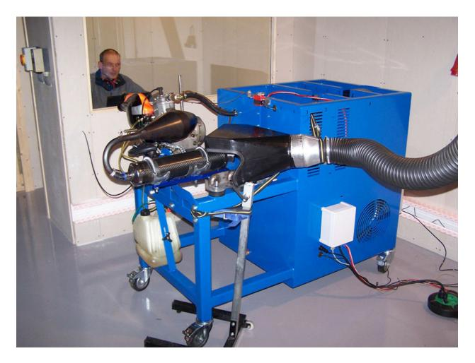
Many kart manufacturers and motor builders will utilize an engine dynamometer similar to the one depicted. These 'dynos' allow karters to simulate the stresses and strain of the engine during competition in a controlled environment, to ensure that the engine package can deliver top-level performance. (PC: Radne)
