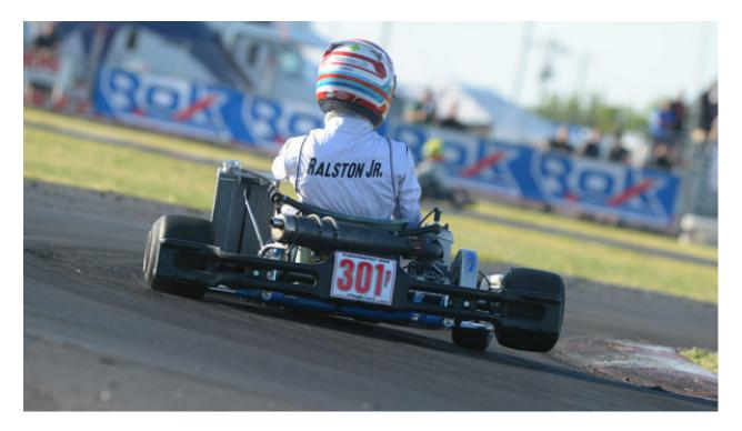
Every modern racing go kart is the result of decades of development by major kart manufacturers. The engineered ability of a kart to 'hike' it's inside rear tire in a corner is the key to the astounding cornering ability most karts produce. Here, a kart demonstrates perfect wheel hike as it travels around a corner. (PC: OnTrack Promotions)
