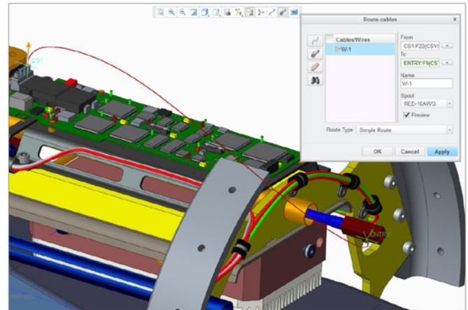
Determine the connections either manually or from logical information. Creo PCX automatically generates a simple path which then enables the user to find the optimum path faster.
