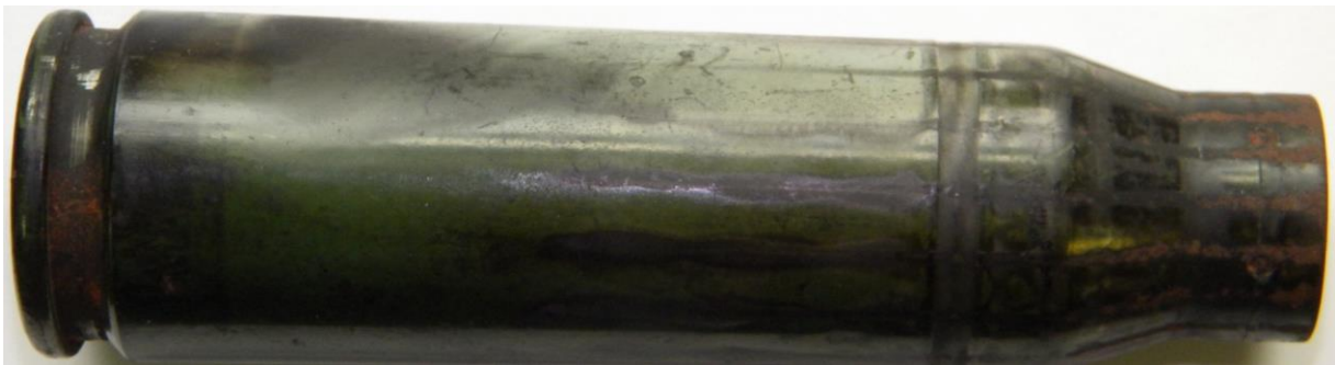
Figure 11: Case Exterior Fired in Fluted Chamber
