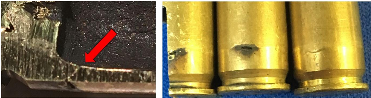
Figure 6: Brass Case Leak Due to Repeated Sizing and Reduced Elongation at Failure
