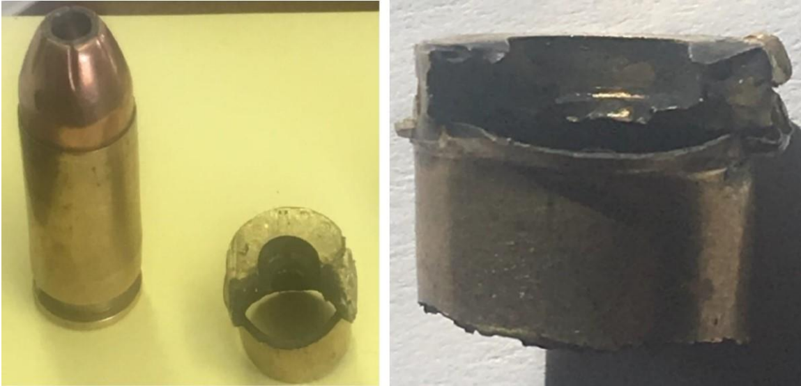
Figure 10: 9x19mm Case Exhibiting Catastrophic Internal Pressures
