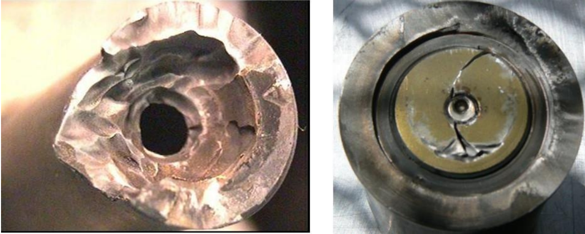
Figure 7: Failures of Improperly Processed Aluminum Cases
