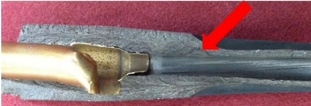
Figure 19: Failed 300 WM Barrel with After-Market External Flutes
