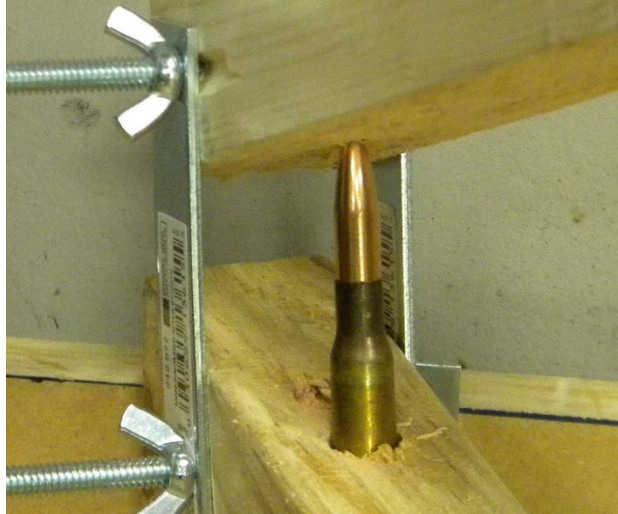
Figure 2: Pressing a Projectile Into the Case Neck
