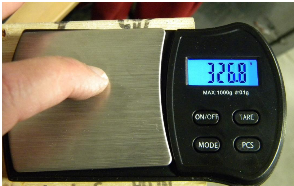
Figure 3: Push Force Measurement
