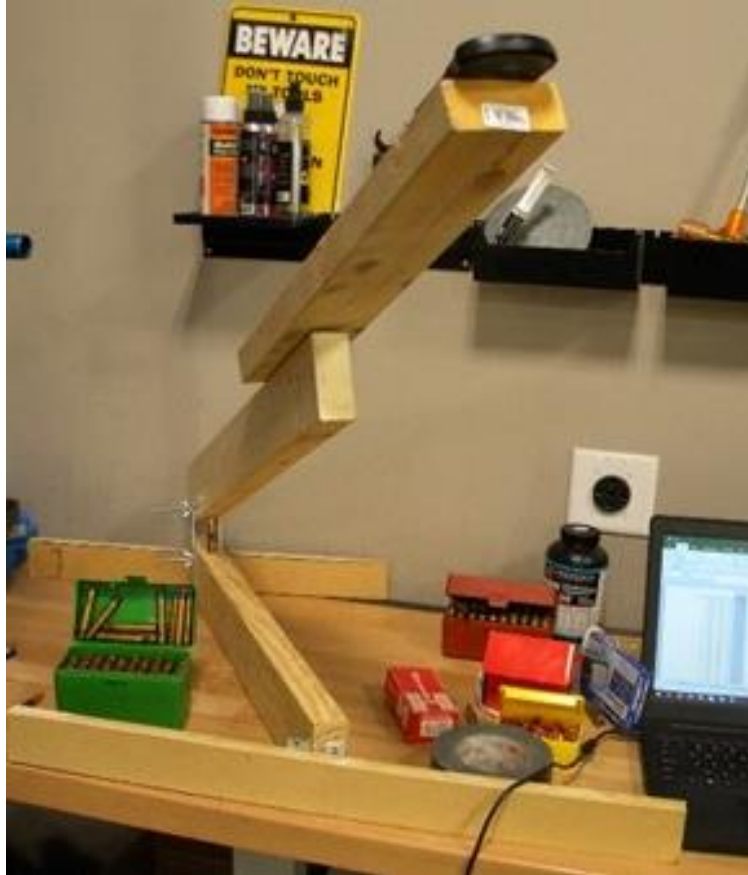
Figure 1: Bullet Press Assembled on Test Bench
