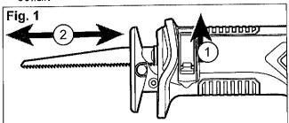
2. Release the lever and the spring loaded mechanism will clamp the blade firmly in place.
