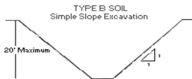
Figure 4 - Normal Sloping configuration for a “type B soil”.
