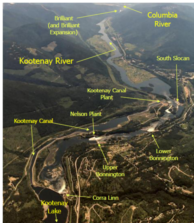
Figure 2. Lower Kootenay River Dams (from International Kootenay Lake Board of Control – International Joint Commission – IJC).
