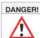
This message denotes the most serious specific hazard. The sign will be displayed on the machine in areas of potential hazard.
