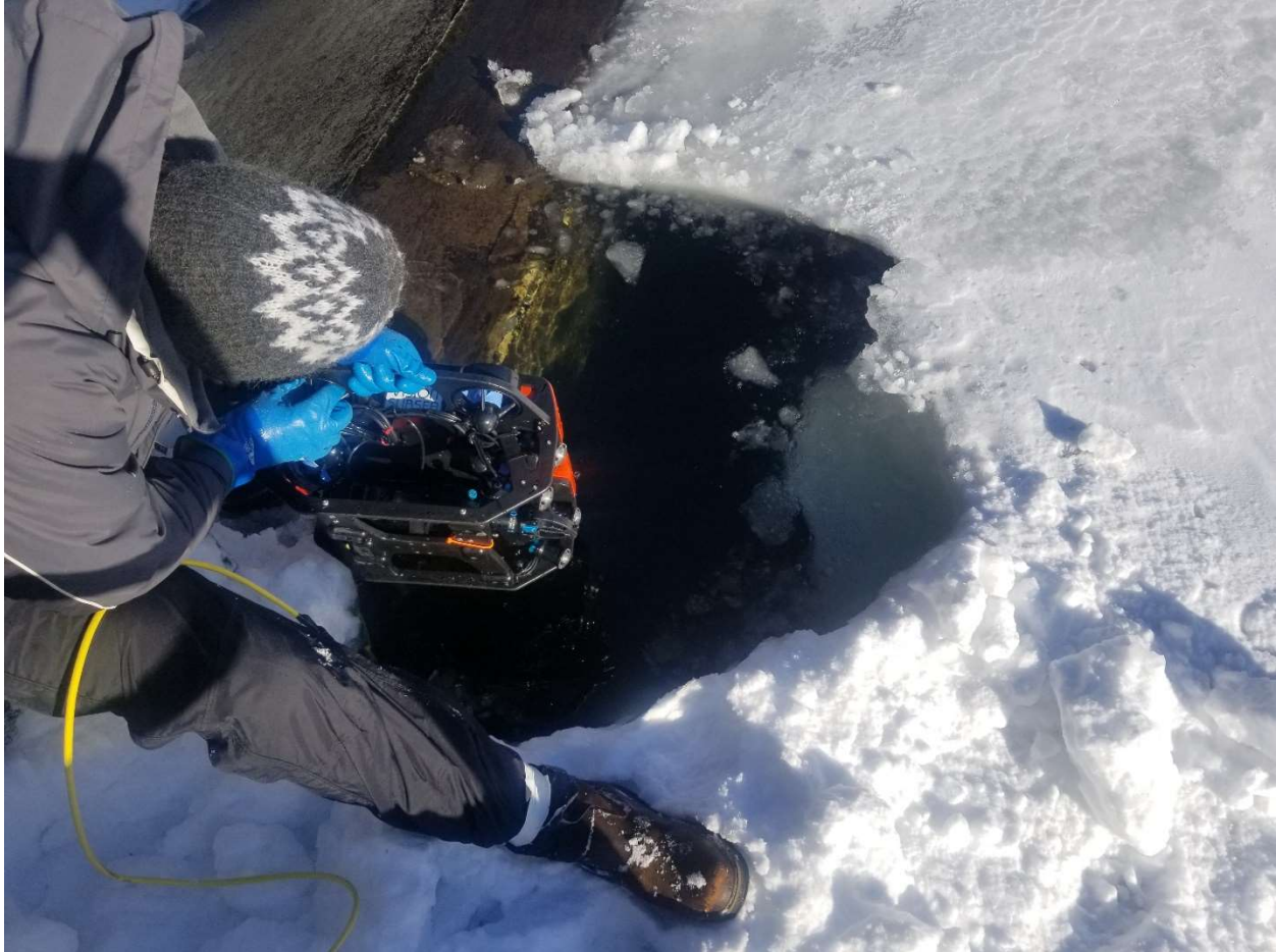
ROV launch into reservoir at spillway
