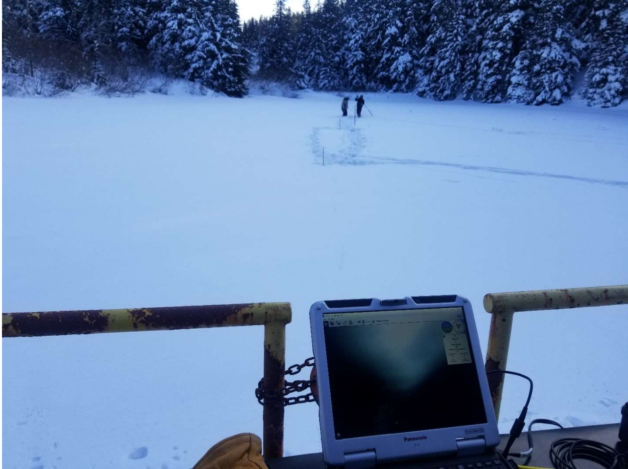
Conducting sounding and sediment level measurement's moving south from dam well
