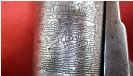
The cylinder scene depicts a city with a bridge and sailing ships, but also a steam ship. This is obviously supposed to be the Colt "Brooklyn Bridge" roll engraving. Apparently these cheap percussion revolvers were still made up until WW1 for sale in the "Colonies"...
