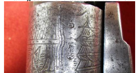
Oddball Belgian Percussion Revolver: The design is similar to the 1850's Colt and Manhattan pocket revolvers however the proof marks date it as having been manufactured after 1893.
