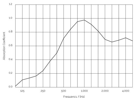
If you are looking for better absorption, we recommend placing 45mm insulation behind the panel. This expands the acoustic solution and will improve the panel's acoustic qualitites.
