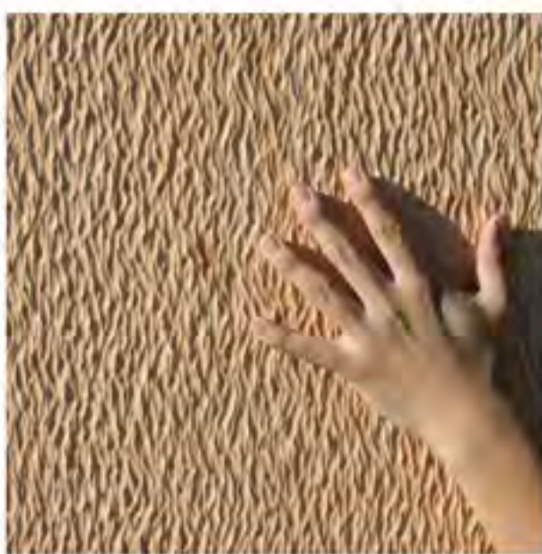
COT 004.25 Pasadena Maple membrane finish PD: 0.115". PT: 0.75". Pattern type: Repeating/ Continuous. Pattern repeats every 24 inches perpendicular to pattern direction and every 48 inches parallel to pattern direction. Pattern direction may be selected in vertical direction or horizontal direction.
