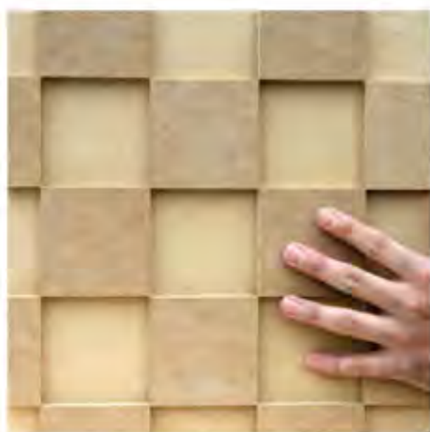
CB 30 Shown in unfinished IDF* PD: 0.375". PT: 1.5". Pattern Type: Repeating. Square sizes are 3" x 3". It is limited to 4'x8' panel only. * - if product is ordered raw IDF then the overall thickness will be 1.25 inches.
