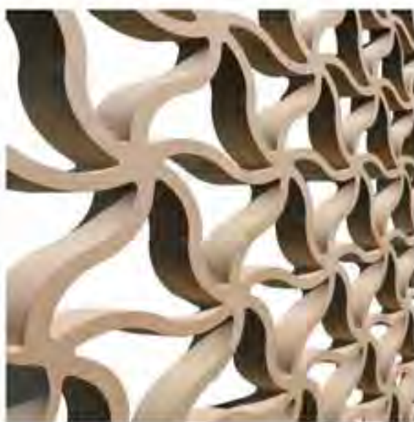
PINWHEEL Shown in unfinished IDF. Pattern Depth: Thru Cut. Panel Thickness: 0.75" up to 1.5". Pattern Type: Repeating. Inside solid area is .25" wide. Border solid area is 0.5" wide. 4'x8' repeating panels only. A border is integrated in the pattern.
