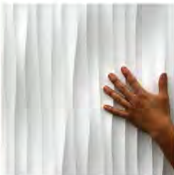
SOT002x2 Snow White membrane finish. PD: 1.0". PT: 1.5". Pattern Type: Repeating/ Continuous. Notes: Pattern repeats every 24 inches perpendicular to pattern direction and every 96 inches parallel to pattern direction. Must be "A-B" panel match for horizontal repeat.
