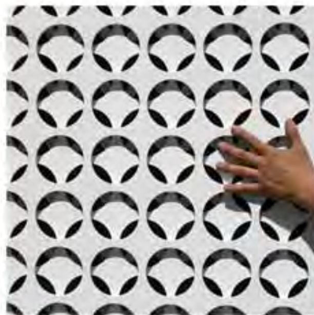
CIRCLE Shown in white paint finish. Double sided pattern. Panel Thickness: 0.75" or 1". Pattern Type: Repeating 3.5" circles on 4" centers. It is limited to 4'x8' repeating panels only. A border is not required.
