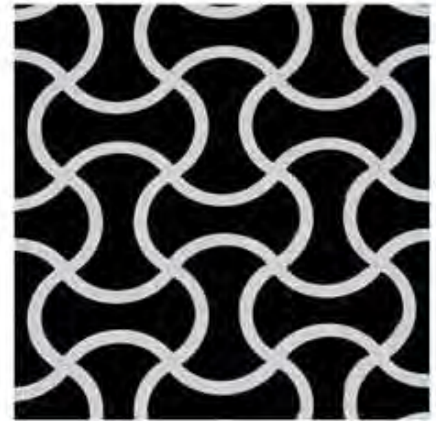
LABRYS 2 Shown in white paint finish. Pattern Depth: Thru Cut. Panel Thickness: 0.75 up to 1.5". Pattern Type: Repeating. All solid areas are 1.5" wide. It is limited to 4'x8' repeating panels only. A border is not required.
