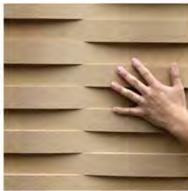
W1202 Shown in unfinished IDF. PD: varies up to 1" depending on panel thickness. PT: 0.75", 1", 1.5". Pattern Type: Repeating 2" band on 12" wave. It is limited to 4'x8' or 4'x 10' panels only.
