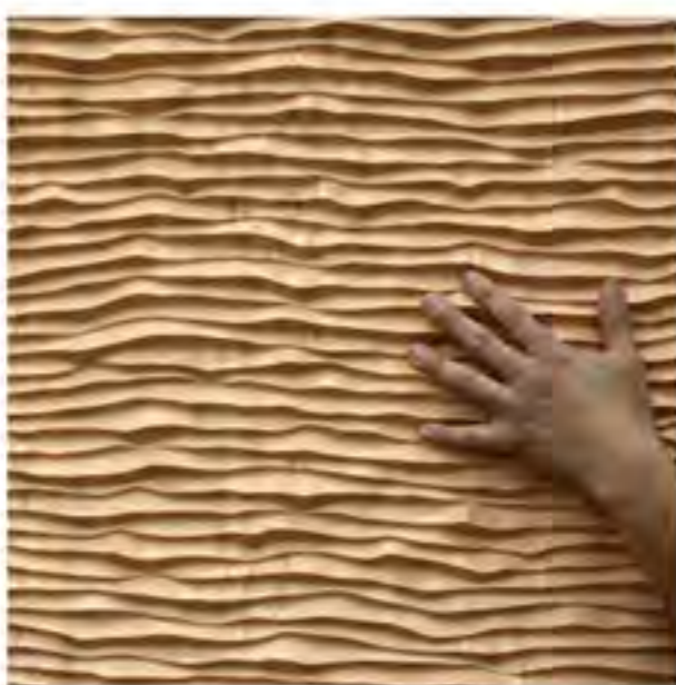
COT 008 Pasadena Maple membrane finish. PD: 0.46". PT: 1". Pattern type: Repeating/ Continuous. Pattern repeats every 24 inches perpendicular to pattern direction and every 48 inches parallel to pattern direction. Pattern direction may be selected in vertical direction or horizontal direction.
