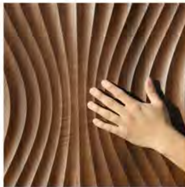
COP 802 Shown in Amati PC membrane finish. PD: 0.3". PT: 0.75". Pattern type: Repeating/Continuous. Pattern repeats every 24 inches perpendicular to pattern direction and every 24 inches parallel to pattern direction. Pattern direction may be selected in vertical direction or horizontal direction.
