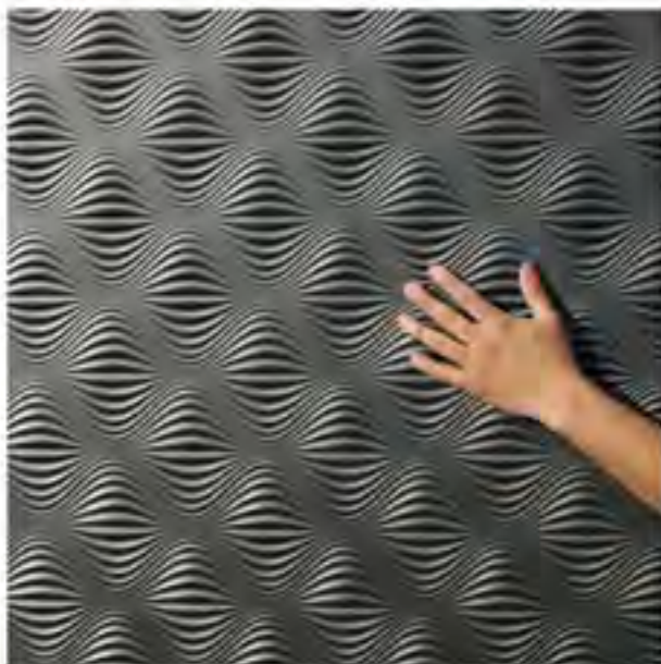
COP 803 Shark Gray membrane finish. PD: 0.3". PT: 0.75". Pattern Type: Repeating/ Continuous. Pattern repeats every 12 inches perpendicular to pattern direction and every 12 inches parallel to pattern direction. Pattern direction may be selected in vertical direction or horizontal direction.
