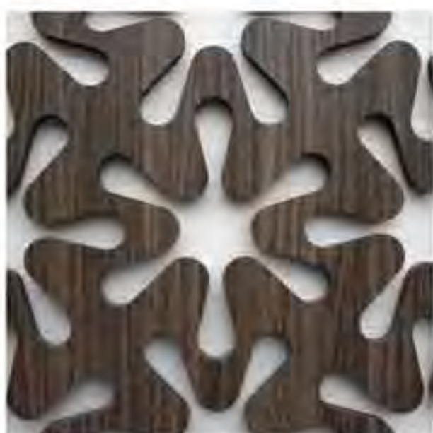
SPLAT Shown in a Lab Designs Laminate overlay. Nominal Panel Size: 48" x 96". Pattern Depth: Thru cut. Panel Thickness: 0.75"-1.5". Pattern Type: Repeating (4' x 8') only. This pattern does not have a border - open edges only. Laminate on both sides is an option.
