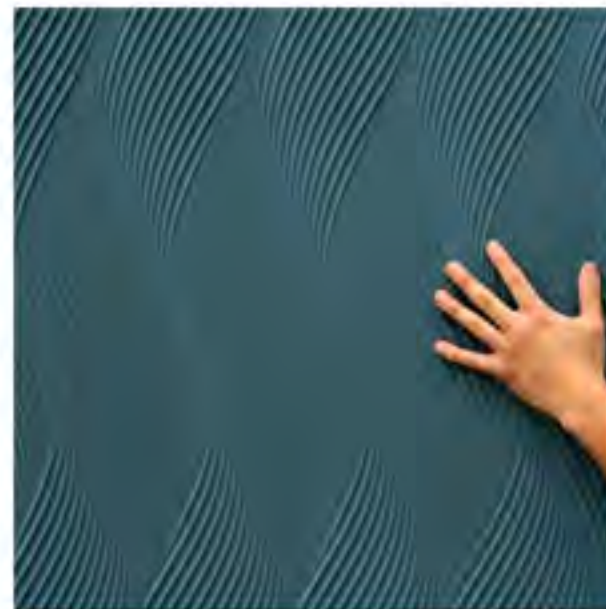
COP 004 Shown in blue colored MDF. PD: 0.3". PT: 0.75". Pattern Type: Repeating/Continuous. Standard panel size is 48" x 96". Pattern repeats every 12 inches perpendicular to pattern direction and every 24 inches parallel to pattern direction - vertical or horizontal.
