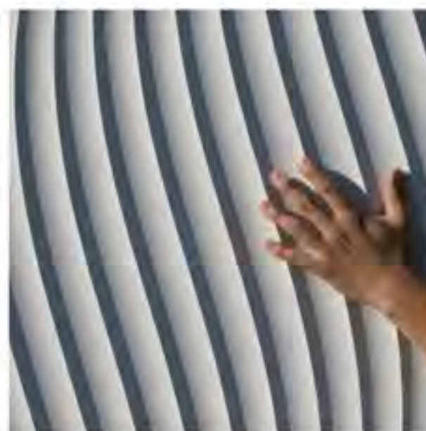
COP 008 Snow White membrane finish. PD: 0.6". PT: 1". Pattern Type: Repeating/Continuous. Standard panel size is 48" x 96". Pattern repeats every 24 inches perpendicular to pattern direction and every 48 inches parallel to pattern direction. Pattern direction - vertical or horizontal.
