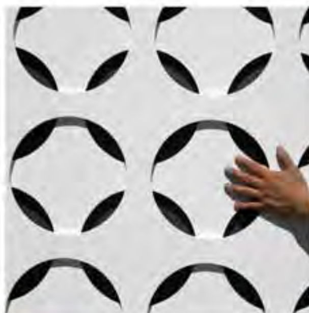
CIRCLE 2 Shown in finish by others. Double sided pattern. Panel Thickness: 0.75" or 1". Pattern Type: Repeating 10" circles on 12" centers. Notes: It is limited to 4'x8' repeating panels only. A border is not required.
