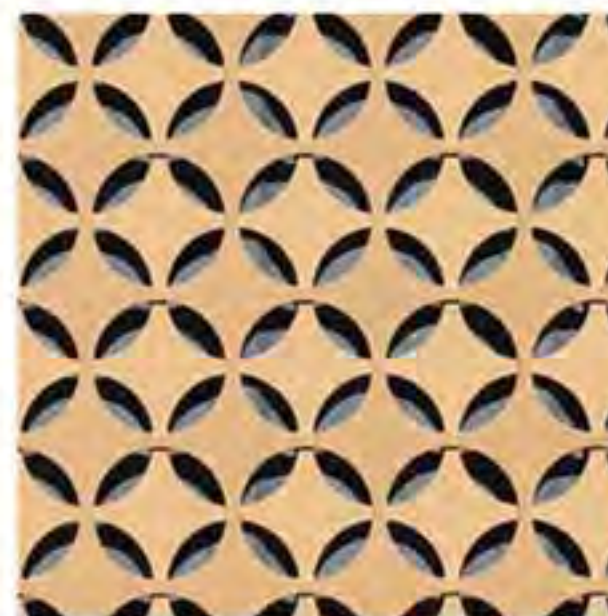
CIRCLE 6 Shown in unfinished IDF. Double sided pattern. Panel Thickness: 0.75" or 1". Pattern Type: Repeating 5.5" circles on 6" centers. It is limited to 4'x8' repeating panels only. A border is not required.
