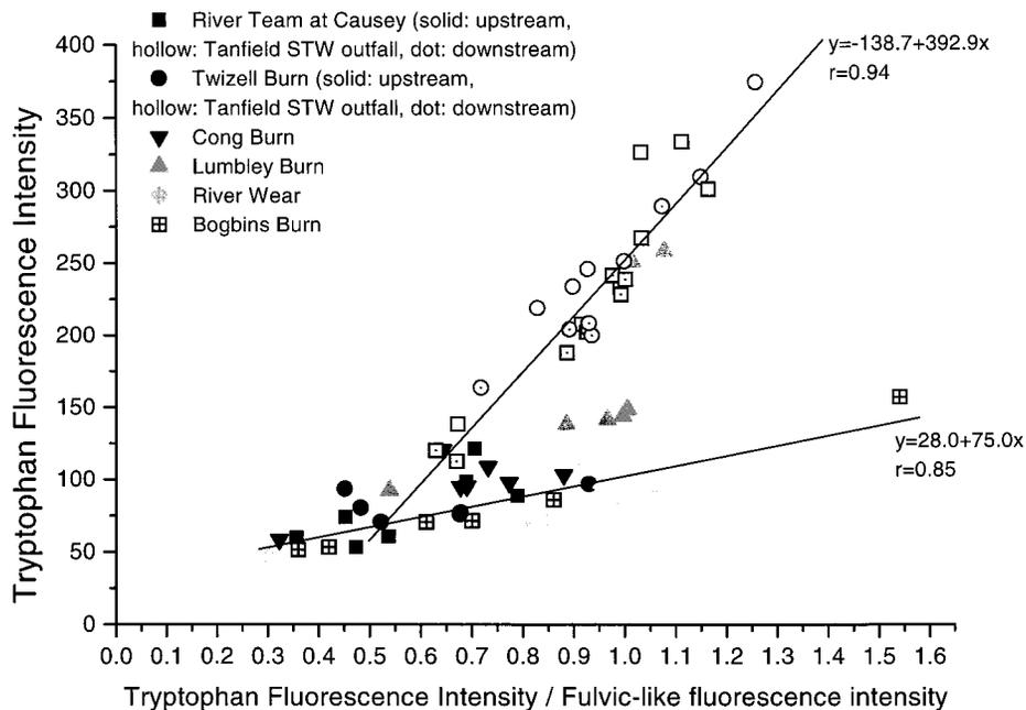
FIGURE 3. Graph of tryptophan fluorescence intensity against tryptophan/fulvic-like fluorescence intensity. The two trend lines are linear regressions fitted to (i) River Team and Twizell Burn STW impacted samples and (ii) all other samples except two Lumbley Park Burn outliers.
