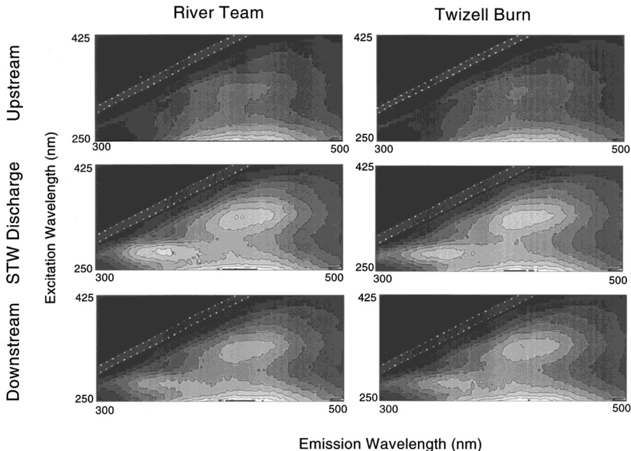
FIGURE 2. Typical fluorescence EEMs for the River Team (East Tanfield STW) and Twizell Burn (Hustledown STW) showing upstream, discharge, and downstream EEMs. Fluorescence intensity is scaled from 0 to 300 intensity units with contours every 30 units; contour labels are omitted for clarity. Note both increased intensity of peaks A and B at the discharge and downstream. Data are from samples taken on the July 4, 2000.
