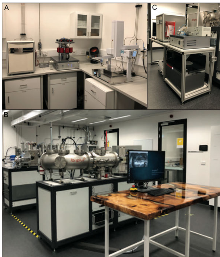
Figure 1 The Chronos ^{14}\text{C} Carbon-Cycle Facility at the University of New South Wales. Panel A: Elemental analyzer with Carbonate Handling System 2 and Automated Graphitisation Equipment 3. Panel B: The MIni-CARbon DAting System (MICADAS) with New Zealand ancient kauri workstation at the University of New South Wales. Panel C: Elemental analyzer coupled to an isotope ratio mass spectrometer with the Gas Interface System.
