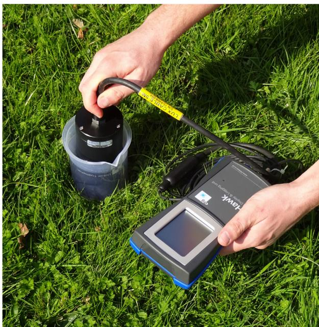
**Fig. 7.** Instantaneous assessment of faecal contamination in drinking water using a tryptophan-like fluorimeter in a beaker and a handheld reader. Note that the sensor operates using UV light and is sensitive to sunlight; hence, the beaker would need to be covered for a reliable measurement.
