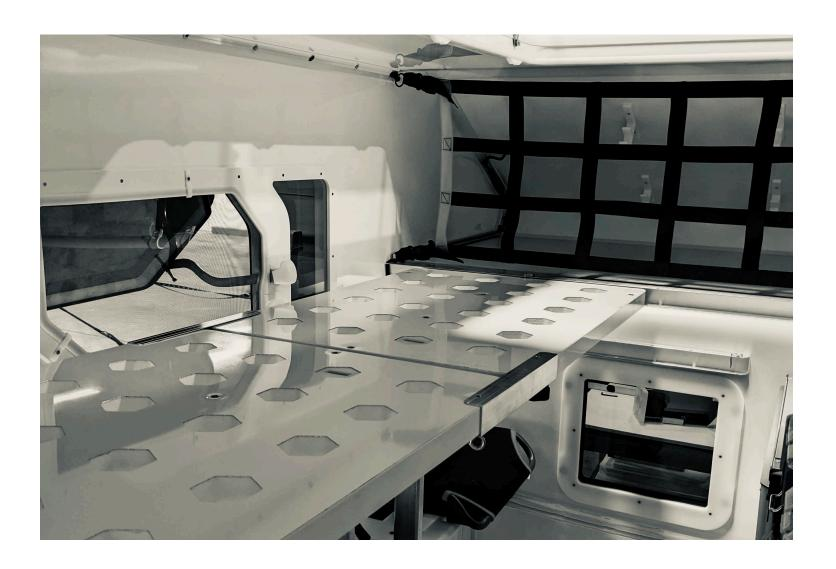
A closer look at the versa panels used to form the beds and tables within this camper. By simple hook lock attachments and mobile leg stands, users find complete functionality and unlimited options for sleeping/living arrangements.
