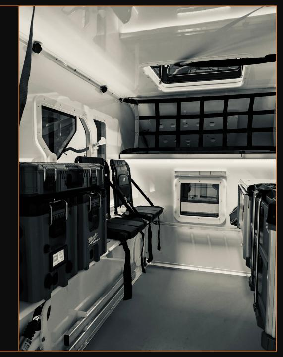
A view displaying 3 seat locations on the left side with a 6 foot long singular bed above. This allows for complete access and usage of storage along the right interior side.
