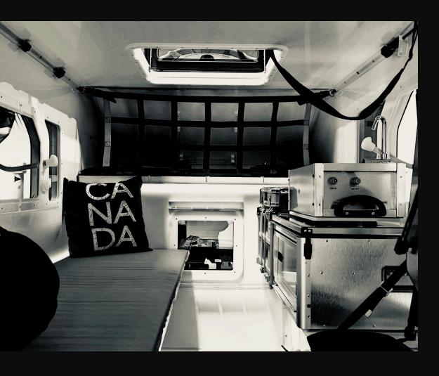
This replica displays a design that allows for single bed sleeping on the left side, with storage of components and 1 seating location on the right. The electrical box is located below the bed allowing for foot room to and from the bed. The overcab displays open options for multiple uses.
