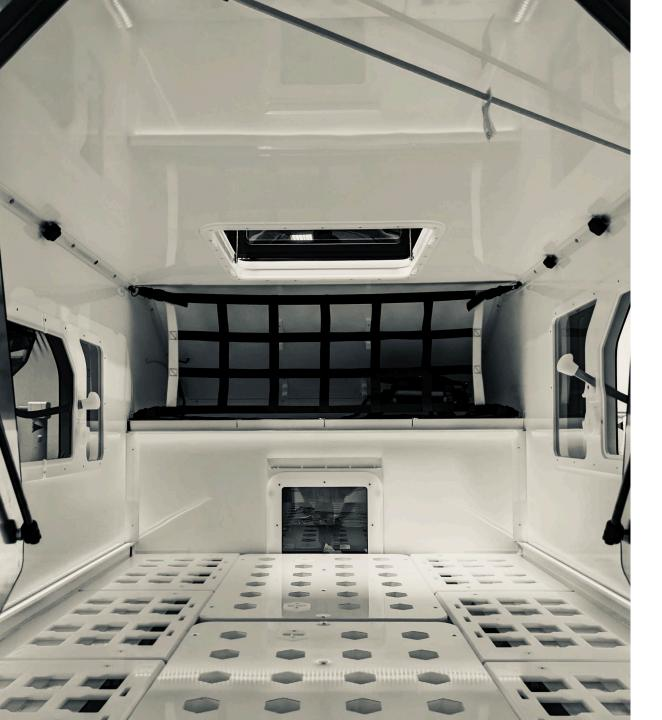
A full size bed, spanning across the interior of the unit. This allows for a sleeping arrangement that can sleep 2 people comfortably. Storage can be utilized underneath the bed and in the overcab.
