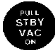
Placard to be located around the LED for the pump inop warning light.
