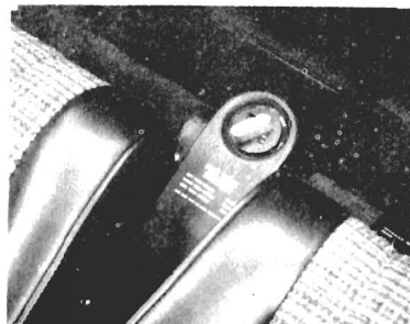
Fig. 1-8 Fuel Selector Valve
