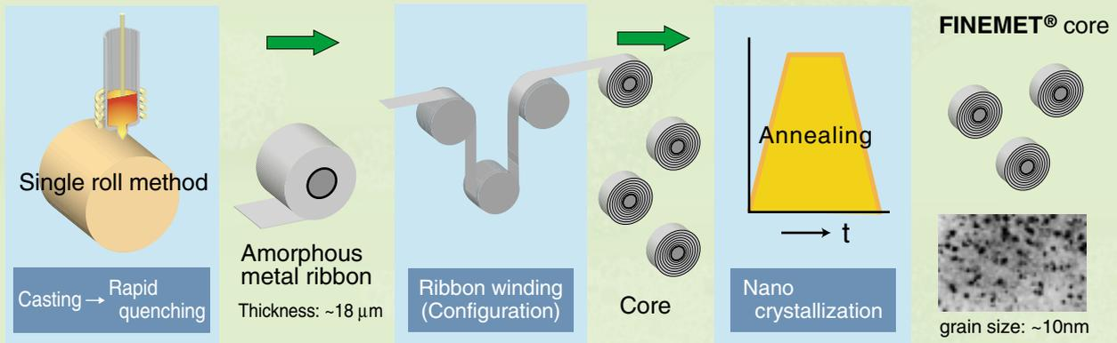
Apply rapid quenching to high temperature melt consists of Fe, as a main phase, Si, B, Cu and Nb.
