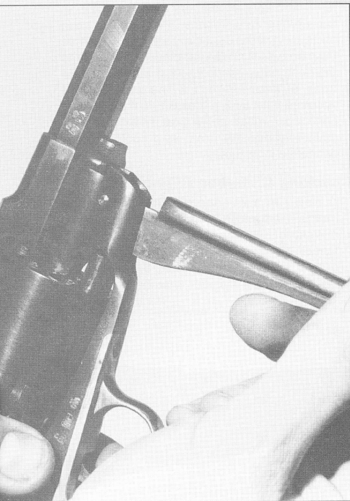
Checking the loading lever for proper alignment with the cylinder chamber.
