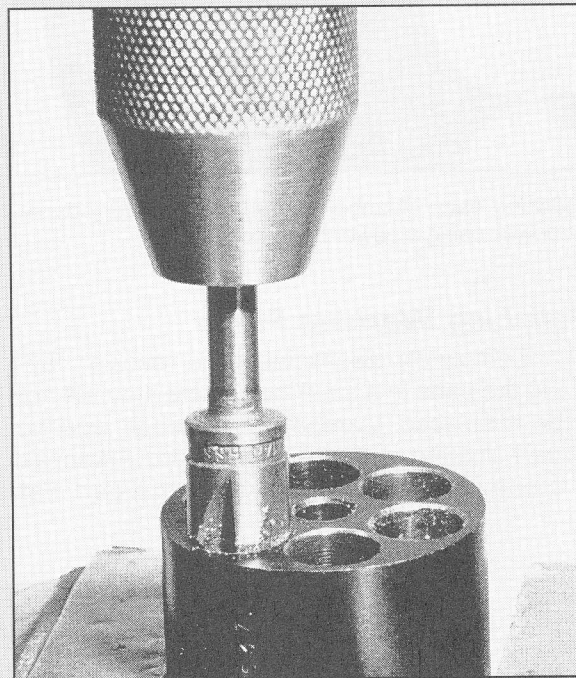
The chambers are being smoothed with a chamfering tool.
