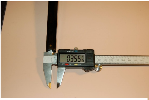
Fig. 2. .355 barrel crown measurement
