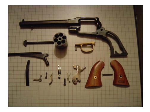
After checking the frame where the action parts are installed and the frame is void of any Burrs or heavy machine marks we will start with the Hammer. It should be polished as shown in the pictures below. Check the firing pin area (face) of the hammer to make sure there are no burrs or other things that may cause the hammer to fail where it enters the frame.
