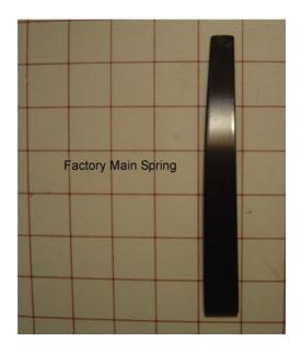
The next step is strictly voluntary. Remingtons have a tendency to have a very heavy trigger pull. To lighten that pull, we will now take the factory installed Main Spring and reduce the sides to make for a smoother Hammer Pull. We want to hour glass the Main Spring, that is remove a little of the metal on the sides to get the desired weakened hammer pull. Ideal is right at 4 lbs of pull. A 4 lb hammer pull will still be strong enough to ignite the Percussion Caps.
