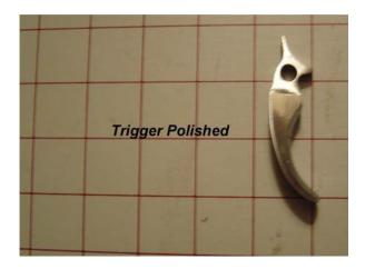
We will now use our Dremel Tool with Stone and remove metal from the left side of the Trigger / Bolt Spring... go easy, you just want to remove a small amount of metal to give the trigger spring the look of a half hour glass. Polish the trigger Spring and insure the bolt side of the Spring (Right Side) is smooth and void of Burrs. Install the Bolt and the Trigger with the Trigger/Bolt Screw into the frame. Install the Trigger/Bolt Spring with the Trigger/Bolt Spring Screw.
