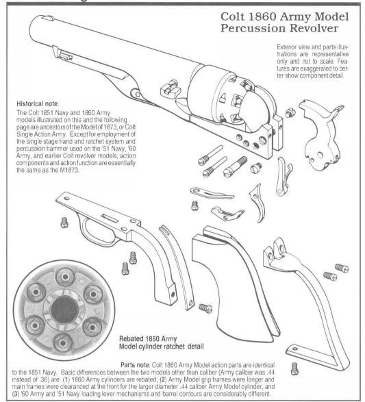
**Figure 8-** Colt 1860 Army Revolver exploded action parts illustration by Heritage-VSP Staff artist is shown for comparison and reference due to action component design similarity. Consult collector publications for additional data on the Colt Army Model of 1860 and other percussion revolvers.
