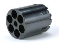
The cylinder chamber mouth on a revolver plays an important part in revolver accuracy in a couple of ways. The job of the cylinder chamber mouth is to guide the bullet from the chamber into the throat of the barrel. The ideal cylinder mouth diameter is about one half a thousandth over the maximum groove diameter of the barrel. In the case of lead bullets, it can be up to .001" smaller than the bullet diameter with decent results. If the
