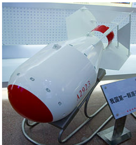
Fig. 4a. The first Chinese Atomic Bomb (mockup). It is rather obvious that it looks like “Fat Man”, although the fissile material used is U-235 and not Pu-239.
