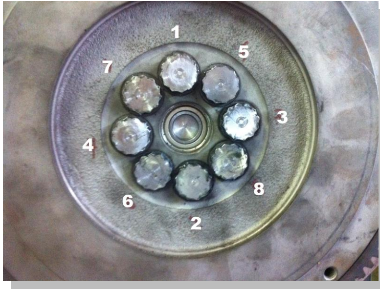
Figure 1 Flywheel torque sequence
