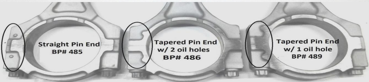
Free-Floating w/bushing - 8mm bolt
