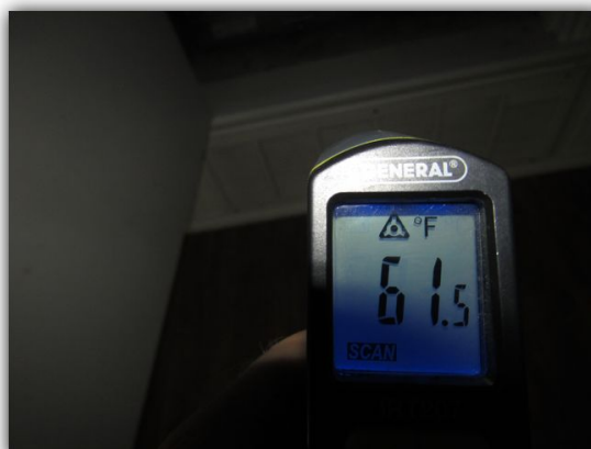
Average temperature between registers and return for home cooling was + 14 degrees.
