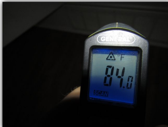
Average temperature between registers and return for Home heating was + 38 degrees.
