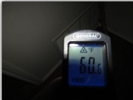
Average temperature between registers and return for Mater Suite Cooling was + 16 degrees.
