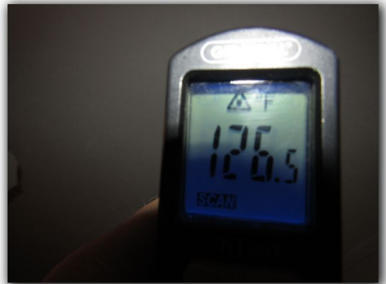
Average temperature between registers and return for Master Suite Heating was + 49 degrees.
