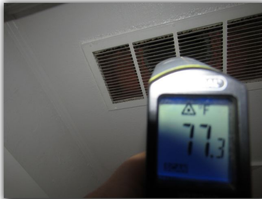
Average temperature between registers and return for Master Suite Heating was + 49 degrees.
