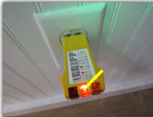
All of the two pong outlets and most of the three pong outlets are on a two wire system with no ground
