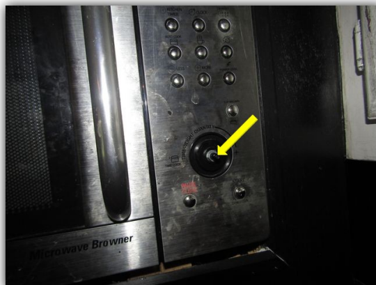
Appears microwave is missing knob
