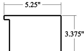
This Trim is used as vertical casings for Windows and Doors and as a transition trim in cases where siding is terminating into something other than a corner or casing.
