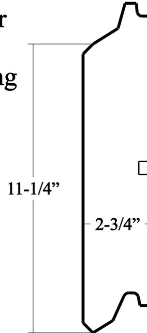
Siding is produced in 12' lengths and each end has a concrete factory edge. For runs shorter than 12', siding can be cut down at the jobsite to the length needed.
