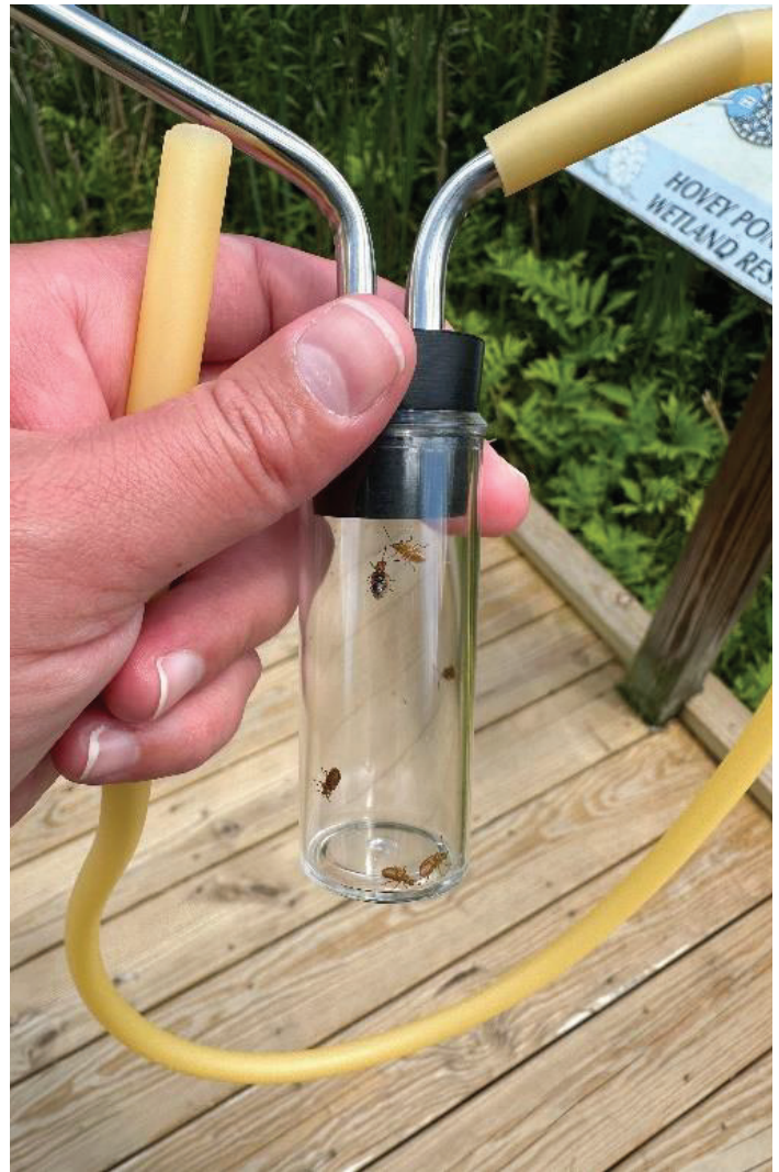
This is an aspirator used to collect beetles by sucking air through an apparatus of metal and rubber straws.
