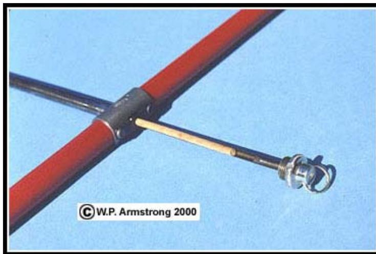
Close-up view of the increment borer, showing the slender wood core that is extracted from the trunk. The core is sanded and treated with a wood oil to make the rings more distinct. Since the rings are so close together, they must be counted under a dissecting microscope.
