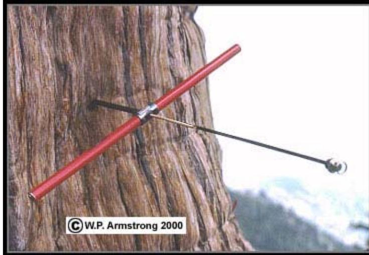
The increment borer removes a small cylinder or core of wood from the tree trunk. By counting the thin bands (annual rings) on the wood cylinder, the approximate age of the tree can be determined. Often the borer does not reach the center of the trunk, so the total number of years must be extrapolated from the radius of the trunk. The radius ( $r$ ) can be determined from the circumference of the trunk ( $C=2\pi r$ ), or from special tape measures that give the diameter directly.
