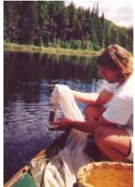
Using Plankton Net to Collect Algae Samples
