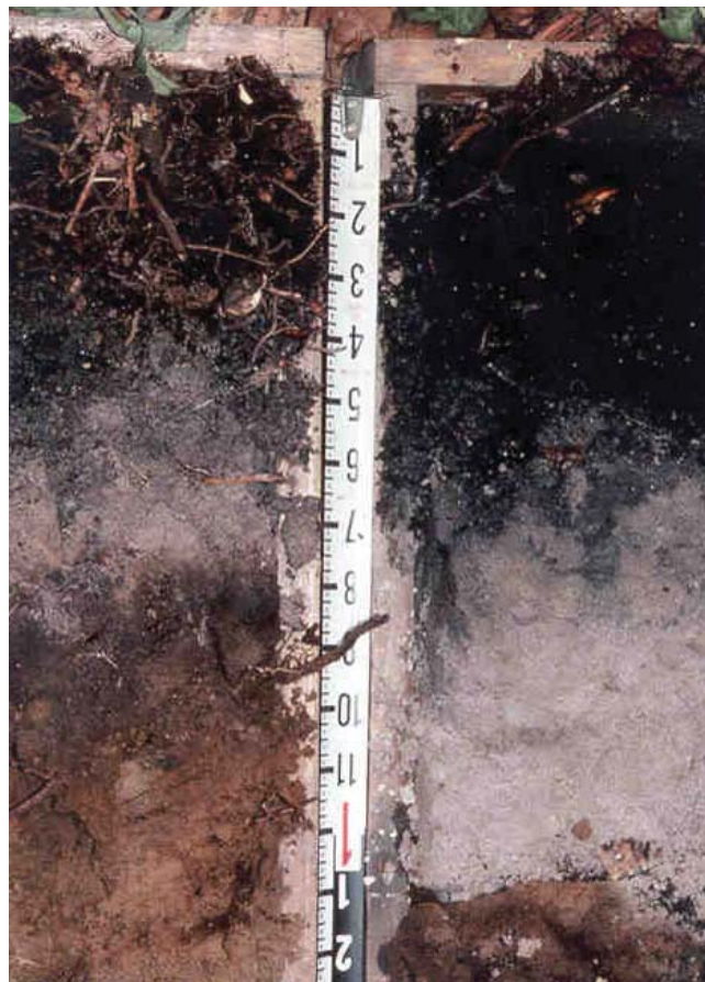
Figure 26.—Indicator S8 (Polyvalue Below Surface, on the right) and Indicator S9 (Thin Dark Surface, on the left). Organic matter has been mobilized and translocated. A spodic horizon is not required but commonly occurs in soils with these indicators. Scale is in inches.
