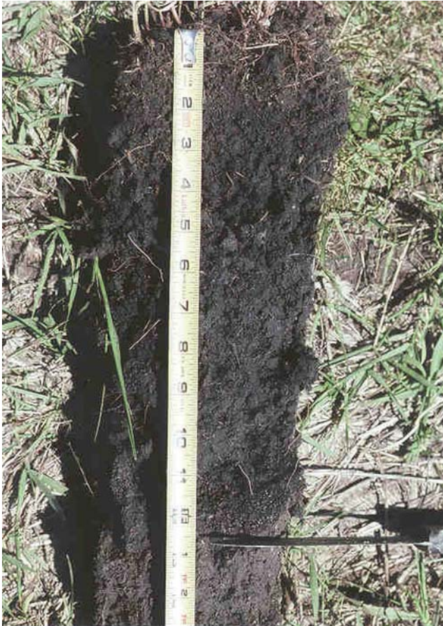
Figure 38.—Indicator F13 (Umbric Surface). This umbric surface is about 20 cm thick. Scale is in inches.
