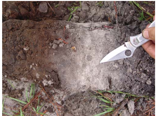
Figure 23.—Indicator S6 (Stripped Matrix). Diffuse splotches, such as those shown in this photo, are a requirement.
