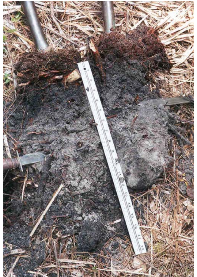
Figure 1.—The field indicators are to be used to delineate hydric soils. The soil on the right is hydric; the Indicator S6 (Stripped Matrix) starts at a depth of about 14 cm. The soil on the left is nonhydric; the Stripped Matrix starts at a depth of about 18 cm.
