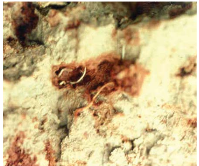
Figure 46.—Sharp boundaries, such as those shown here, may indicate that the redoximorphic features are relict.
