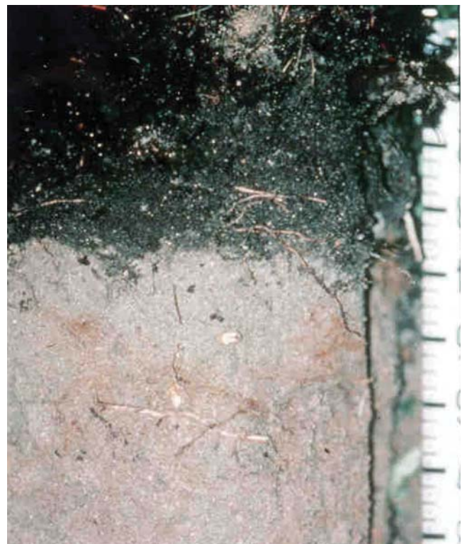
Figure 21.—Indicator S5 (Sandy Redox). The redox masses occur below a depth of about 10 cm. Scale is in inches.
