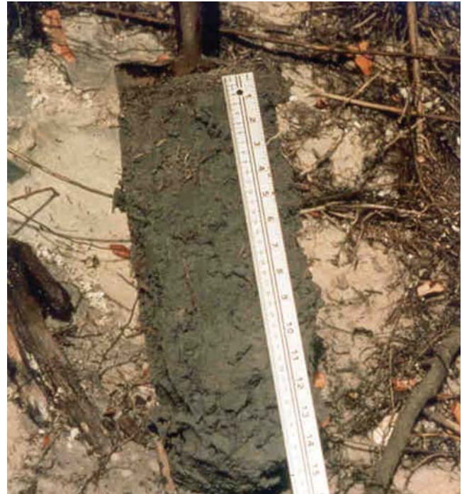
Figure 20.—Indicator S4 (Sandy Gleyed Matrix). The gleyed matrix begins at the soil surface. Scale is in inches (R) and cm (L).
