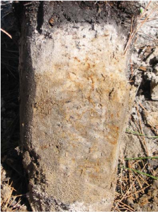
Figure 22.—Indicator S5 (Sandy Redox). The redox masses occur almost to the surface. The soil slice is about 40 cm. Indicator S6 (Stripped Matrix) also occurs in this soil.
