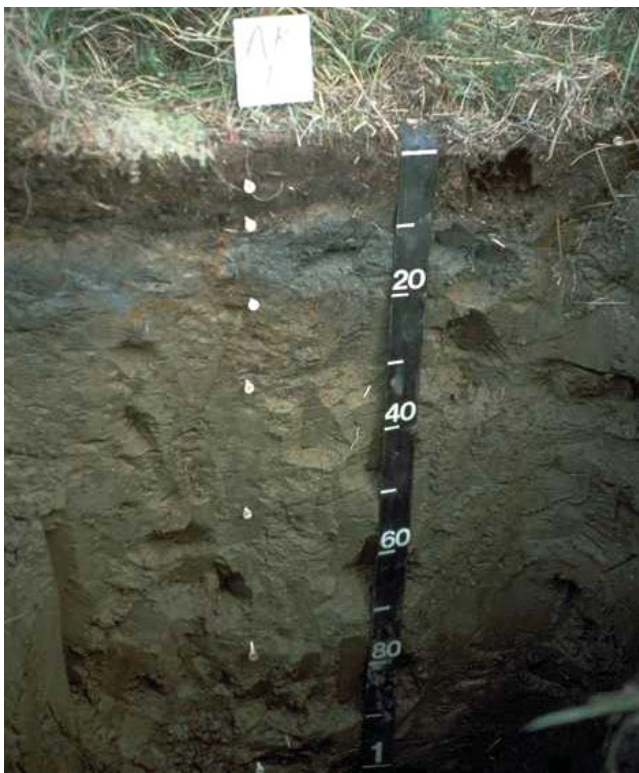
Figure 17.—Indicator A13 (Alaska Gleyed). Bluish band at approximately 20 cm (8 inches) indicates the presence of reduced soil material. The underlying material below 20 cm reflects both the color of the parent material and soil weathering under aerobic conditions.
