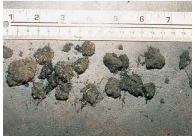
Figure 12: Indicator A6 (Organic Bodies). The individual organic bodies are 1 to 3 cm in size. Scale is in inches (upper) and cm (lower).
