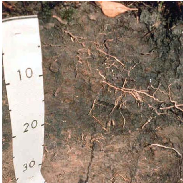
Figure 31.—Indicator F6 (Redox Dark Surface). Prominent redox concentrations occur as soft masses and pore linings. Below the dark epipedon is indicator A11 (Depleted Below Dark Surface). Scale is in cm.
