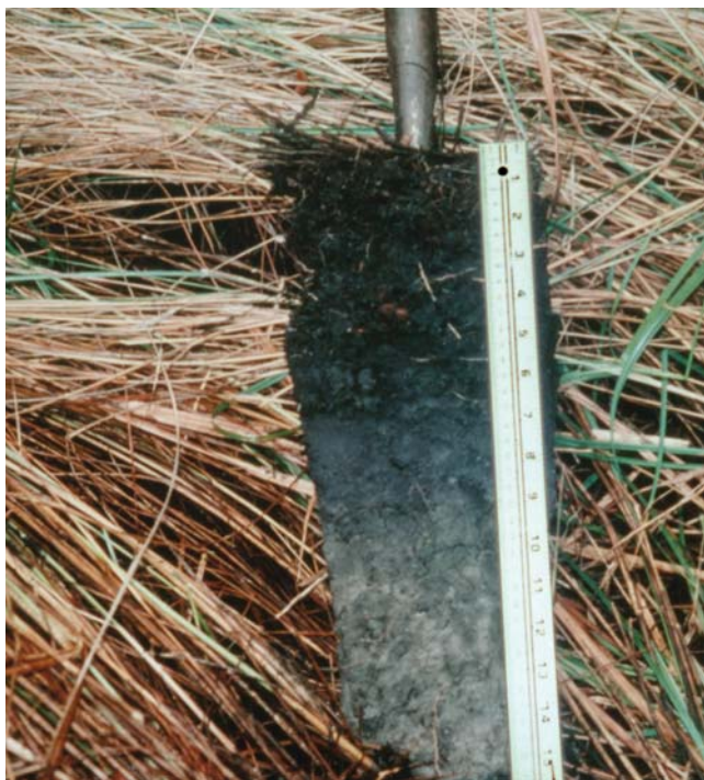
Figure 25.—Indicator S7 (Dark Surface). The dark surface layer is about 15 cm thick. The material below 15 cm meets the intent of Indicator S8 (Polyvalue Below Surface). Scale is in inches.
