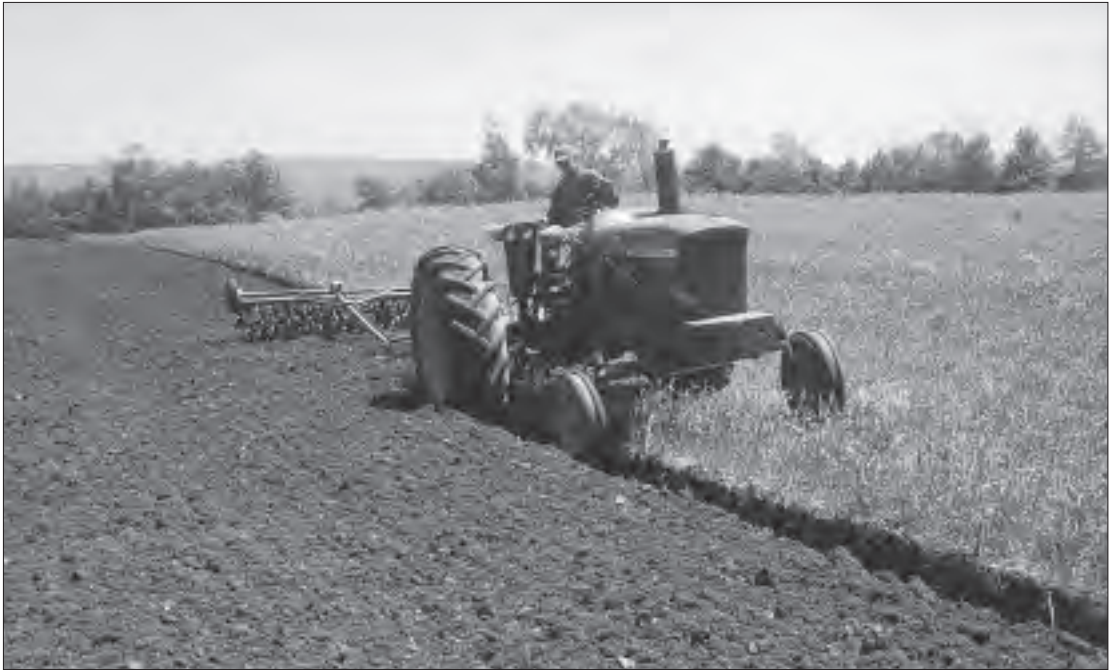
Figure 6.10 Tractor wheels in open furrow during plowing compacts subsoil.
