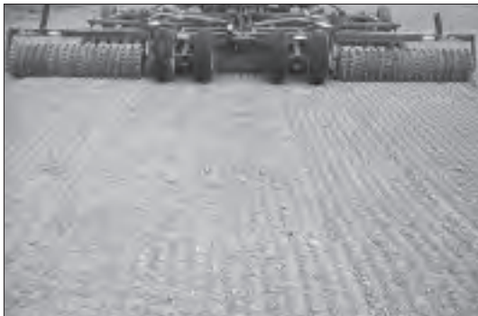
b) Stage 2: Soil is packed and pulverized to make a fine seedbed.
