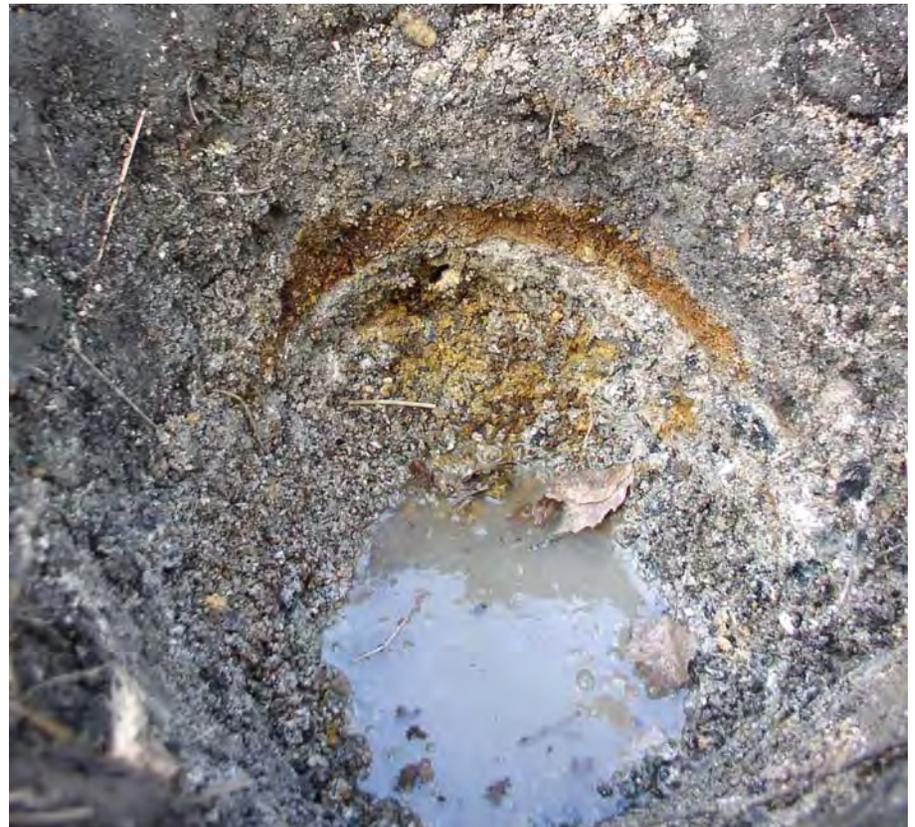
Digging a test pit can reveal the soil horizons and can be used to test the drainage rate of a site.
