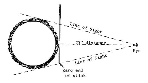
Figure 1. Diameter measurement.
