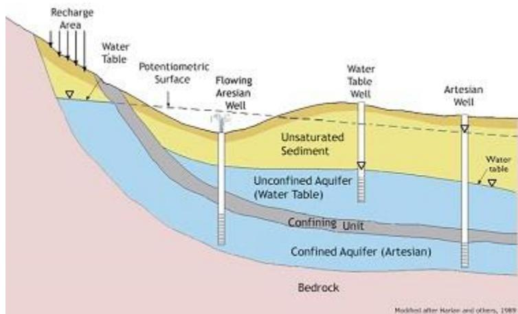
Figure 1. Water table aquifer and an artesian aquifer with flowing and non-flowing wells.
