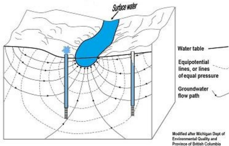
Figure 2. Topographically controlled flowing well in an unconfined aquifer
