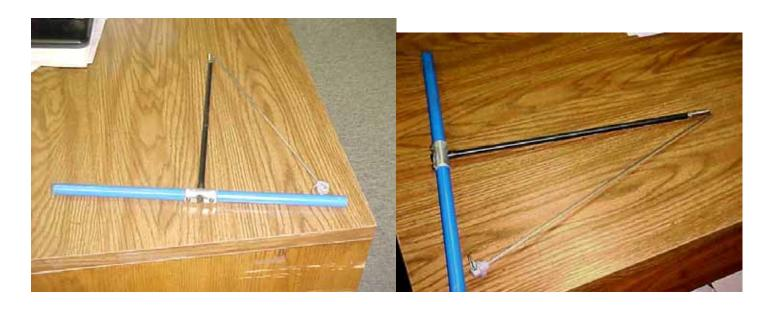
Used to take a core sample of wood from a tree to determine growth rate, age and tree soundness.
