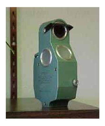
A relaskop can be used as a rangefinder, a clinometer, a dendrometer, an angle gauge, a prism and as a slope correction device.
