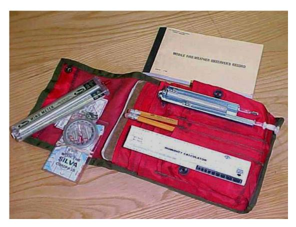
Used to measure relative humidity, wind speed and direction, temperature, and fuel moisture during fire operations.
