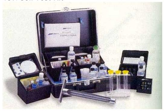
Used to test soil for pH, nitrogen, phosphorus, and potassium levels. Also gives results for soil texture and classification.
