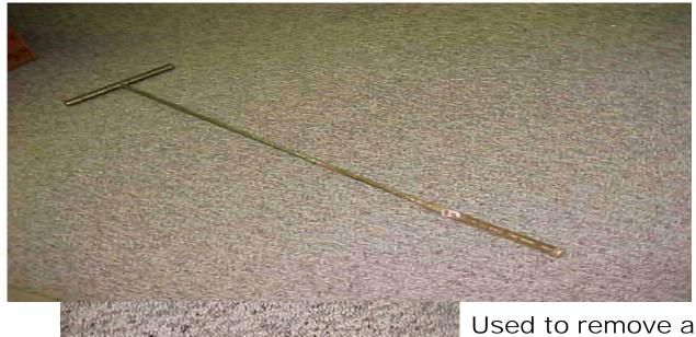
used to remove a soil core sample from the soil to check soil type, conditions and consistency.
