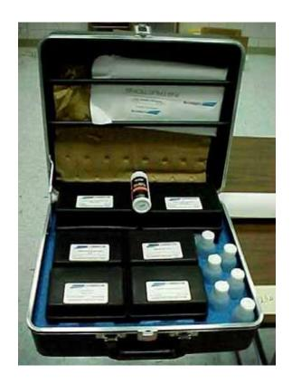
Used to test water for pH and water hardness and to test for levels of nitrogen, oxygen, phosphate, carbon dioxide, and chloride.
