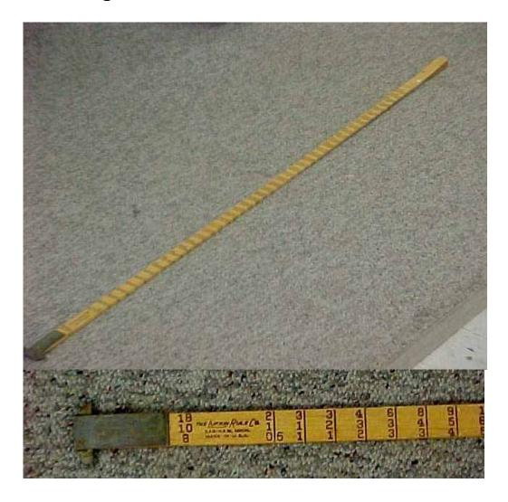
Used in log scaling to determine net volume of raw logs at the saw mill.
