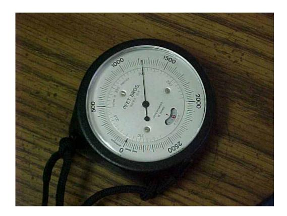
Used to measure elevation.
