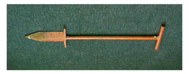
A device used to open and close a planting hole during reforestation.
