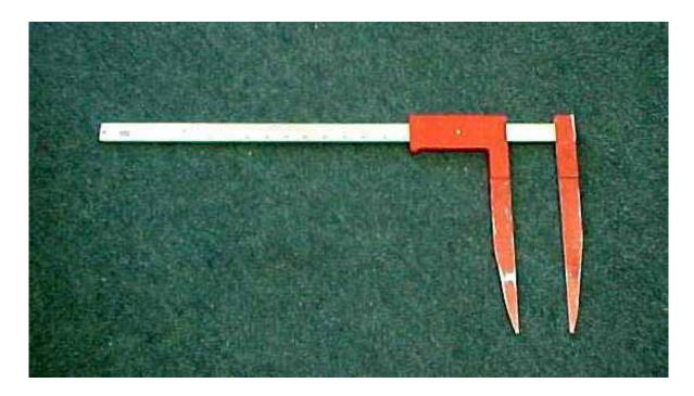
Used for measuring the diameter of trees, logs, and poles.
