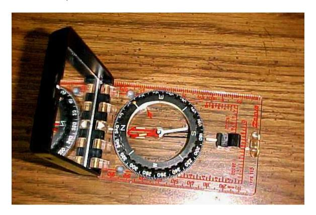
Used to determine which direction is north, to determine the direction of an object or to follow an azimuth.
