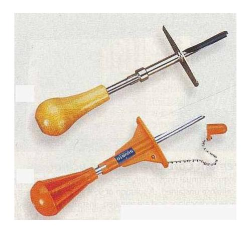
Used to measure the bark thickness of trees. When pressed against the bark, the scale recedes into the handle and the borer cuts out a core of the bark.
