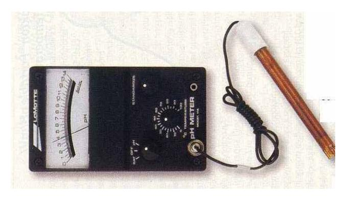
Used to test water and semi-solids for pH value.
