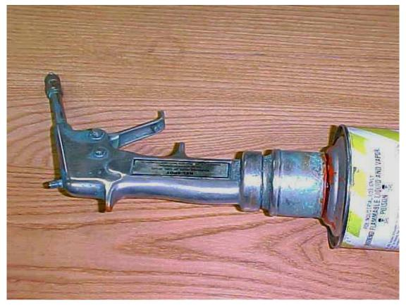
Used to mark timber and timber sale boundaries with paint.
