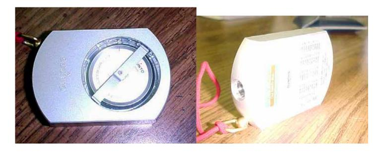
Used to measure tree height and slope.
