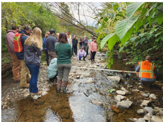
Figure 2 Gale Neale, Stream Program Engineer and Mike Coryat measure the stream channel width at a riffle in Third Brook.
