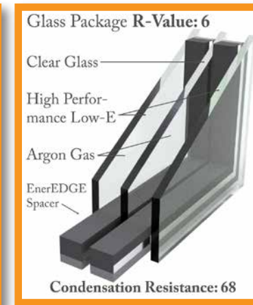
Triple Pane with 2 coatings High Performance Low-E and Argon gas
