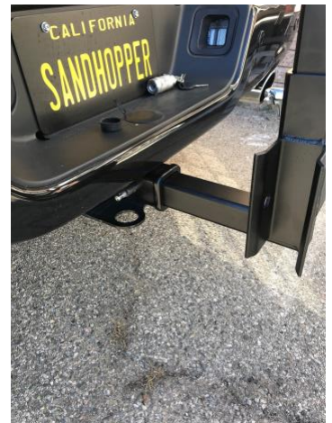
Fig 7. Lift beam & U channel
