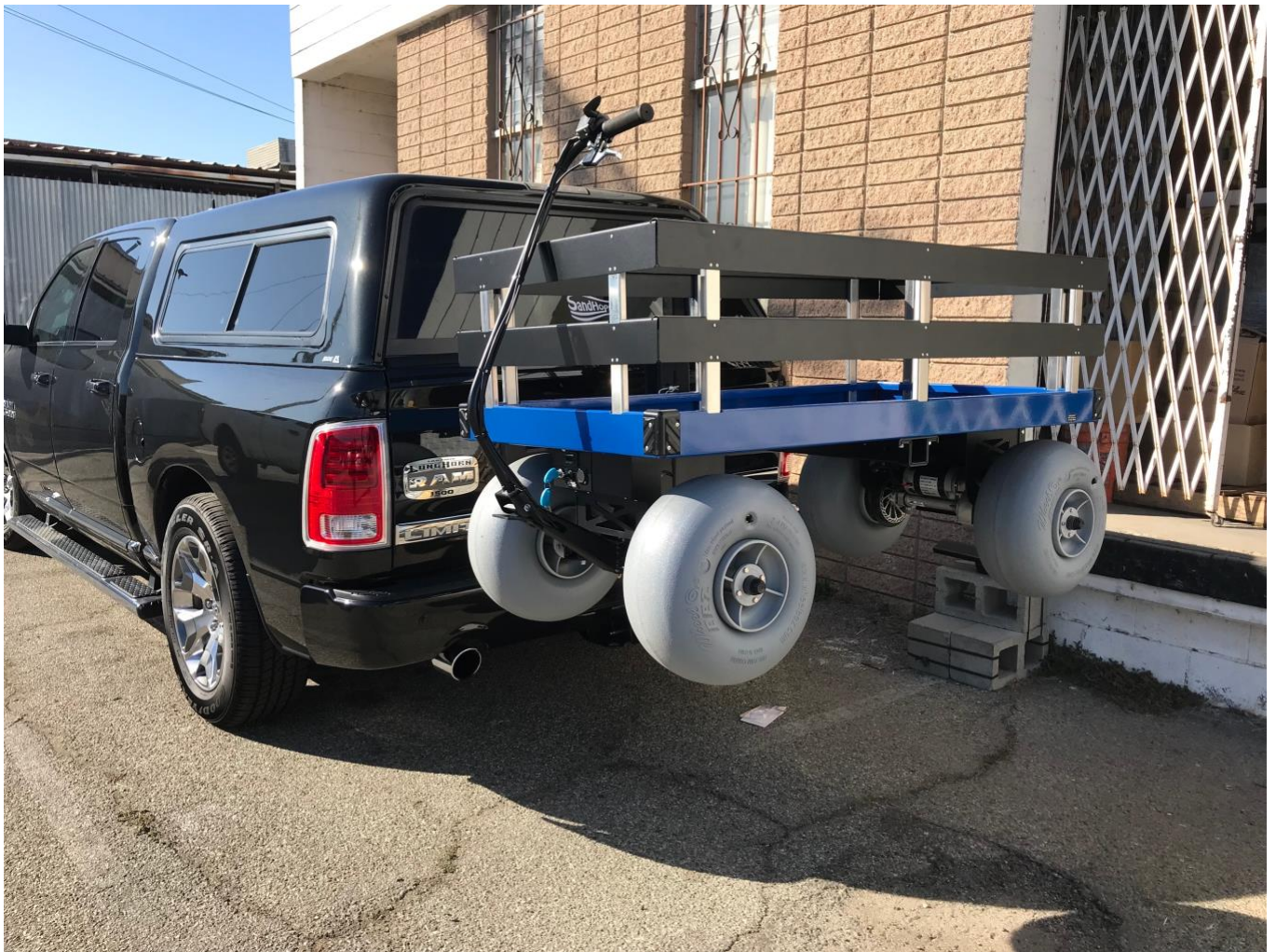
Fig 14. Wagon in locked height (Remove side rails and fold in steering handle and secure). Remove Key switch, check battery straps and any loose objects from the wagon. Check that all 5/8 lock pins are installed properly and retaining clips are installed and secure.
