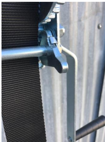
Fig 4. Direction lock Pawl
