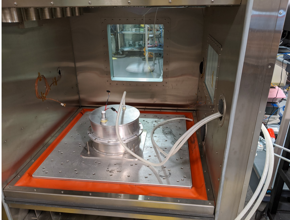
example HALT setup for ACS in T-cell
