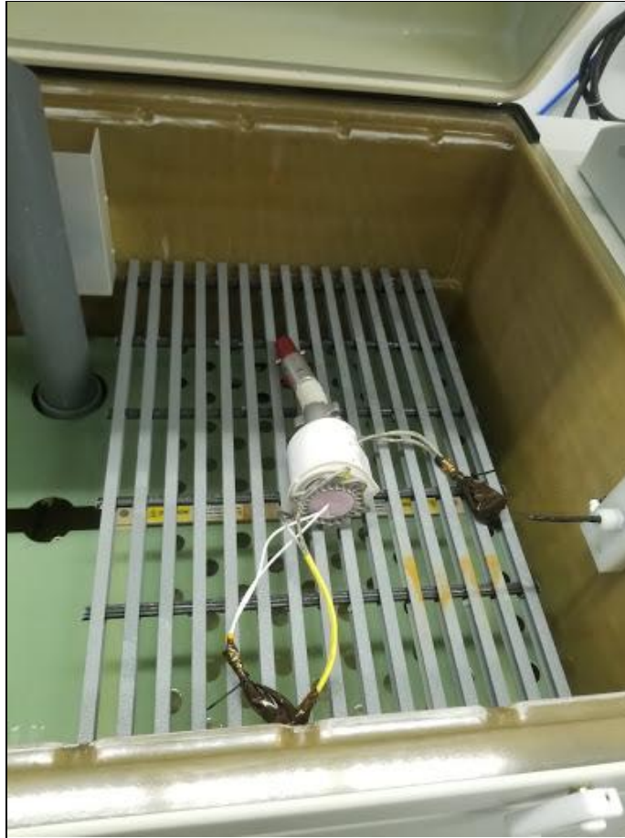
Example DS10 setup in salt fog chamber
