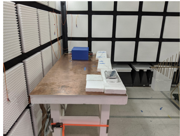
Example of Descent assembly set up in anechoic chamber
