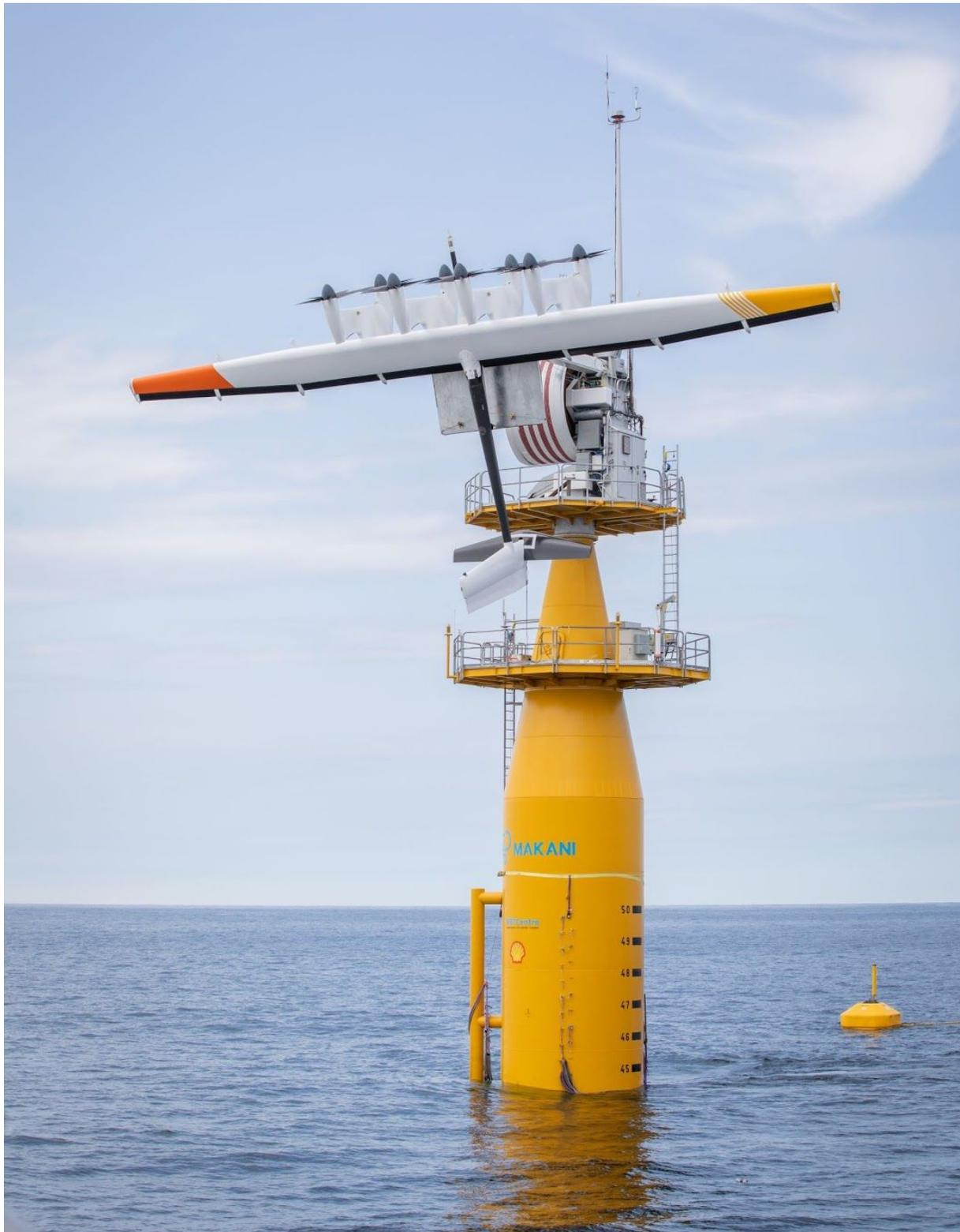
**Figure 13: Photograph of the installed M600 system in the North Sea at the Marine Energy Test Centre in August 2019.**
