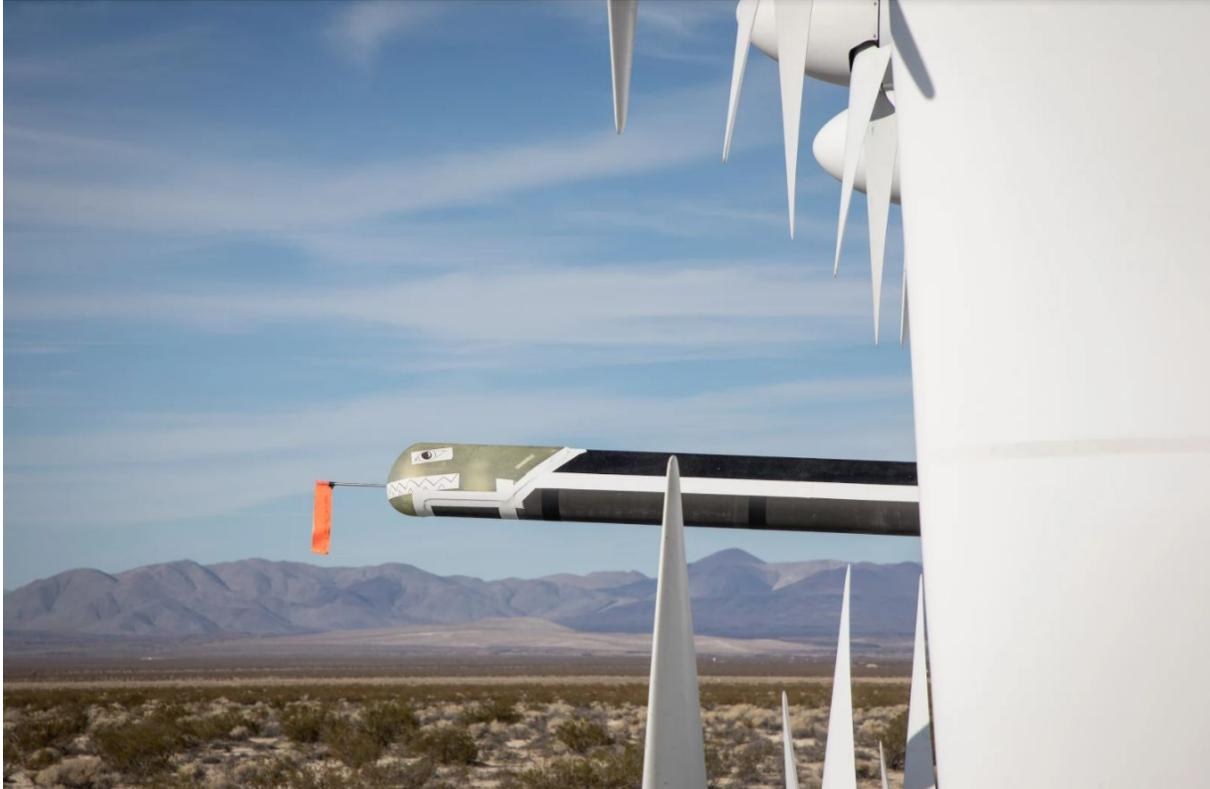
**Figure 19: Profile shot of the mass-balance tube, taken during preflight inspections at China Lake. The pitot tube, covered with a protective orange flag, sticks about 10 cm ahead. The plane of the rotors and the leading edge of the pylons can be seen in this view.**
