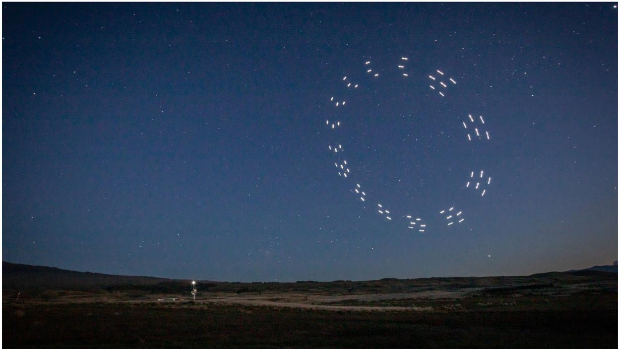
**Figure 10: Makani lighting demonstration for the FAA during a night flight at the Hawaii test site in 2019. The long exposure over a crosswind loop shows the wing tip and tail lights, and the base station tower light, flashing synchronously at 40 flashes per minute. The patterns that appear to be double flashes are, in fact, overlapping successive flight loops.**
