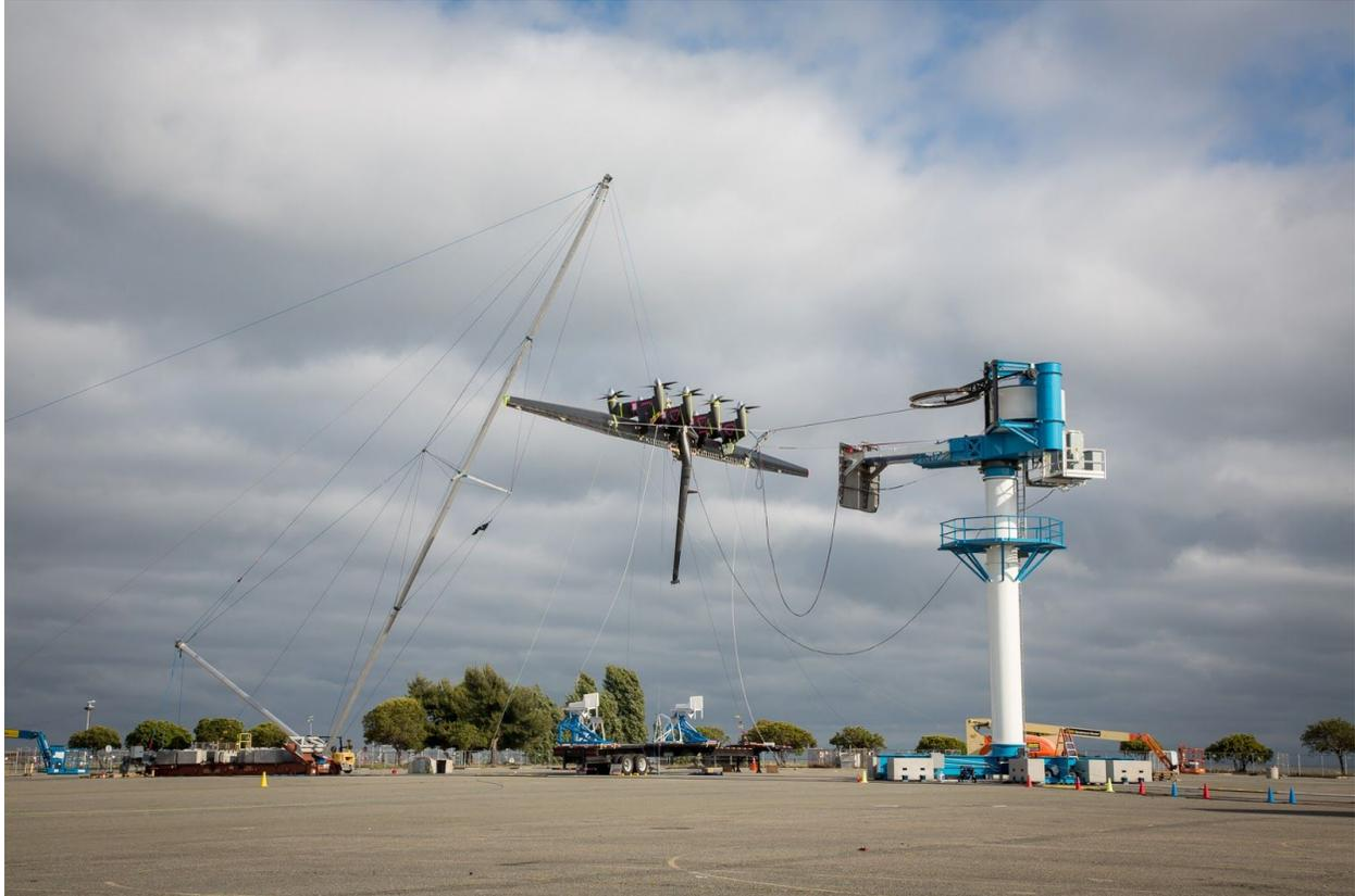
**Figure 2: The first M600 ground station, GS01, and the first assembled kite, SN1, under constraints at the “E-Lot” hover test site in May 2015. In this photo, the kite is still missing major components, including ailerons and an empennage. Most subsystems (including the main wing structure, the motors and the motor controllers) went through a major design iteration before the crosswind-ready kite left the E-Lot in September 2016.**
