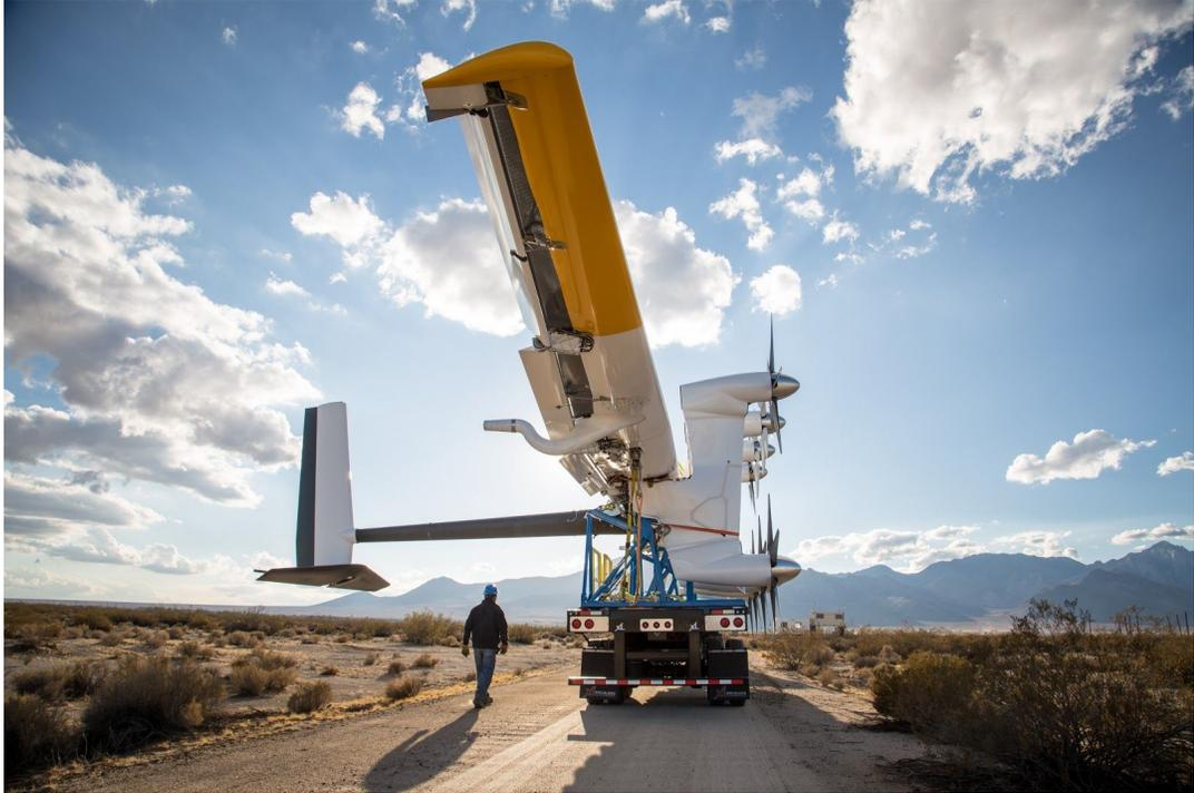
SN2 was the first crosswind-capable airframe and was flown in the test site at China Lake, California. SN2 was lost during hover at the end of flight RPX-06.
