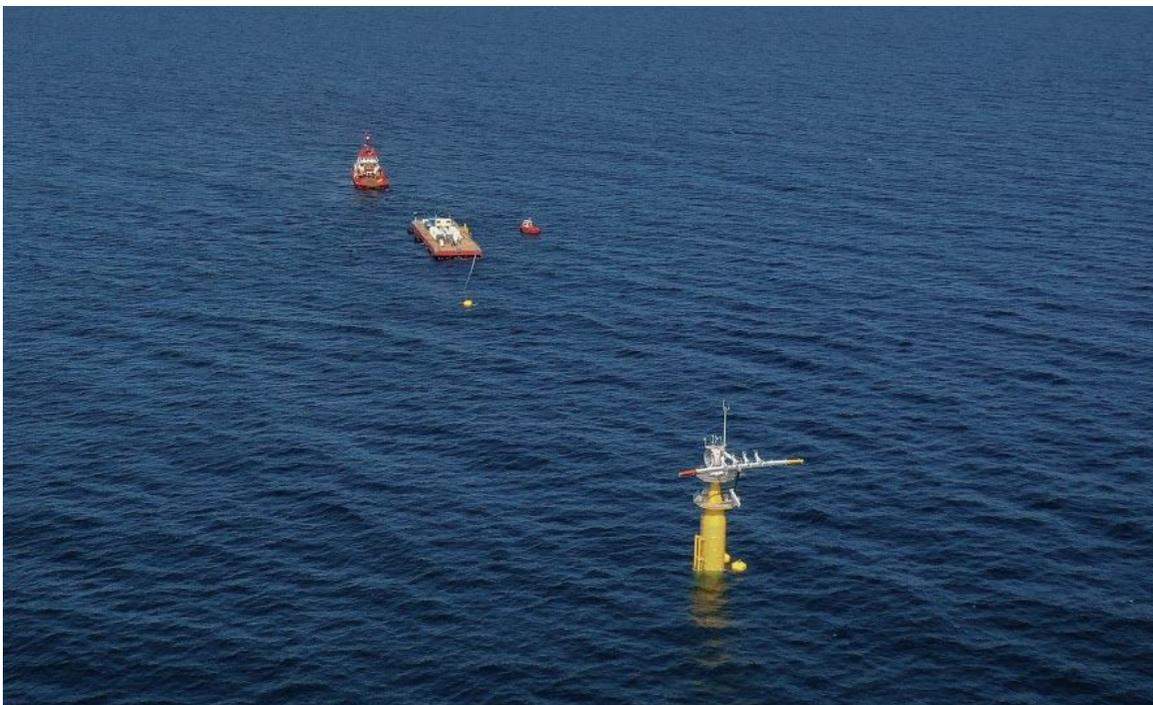
**Figure 12: Norway offshore test site at the Marine Energy Test Centre (Metcentre), showing the barge with the command center and the microgrid containers, and the tug boat for station-keeping (top left).**
