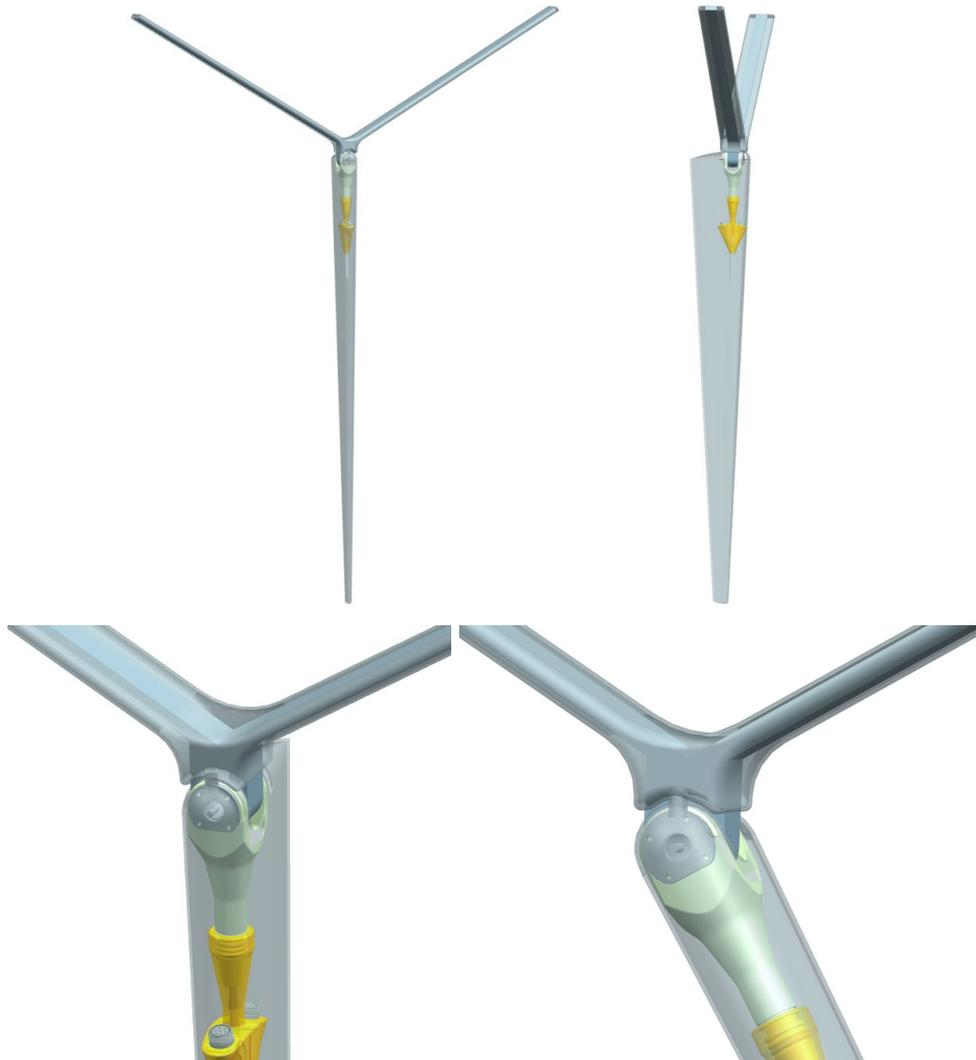
**Figure 9: A CAD mockup of a rigid bridle design. The pitch pivots would be at the wing. The two lower images are close-up views of the roll pivot. Fairings provide (a) drag reduction, (b) protection for the high voltage tether conductors, and (c) an attachment point for a “slack bridle” for passive roll control during hover. The “wishbone” would mate with the ground station cradle for perching.**
