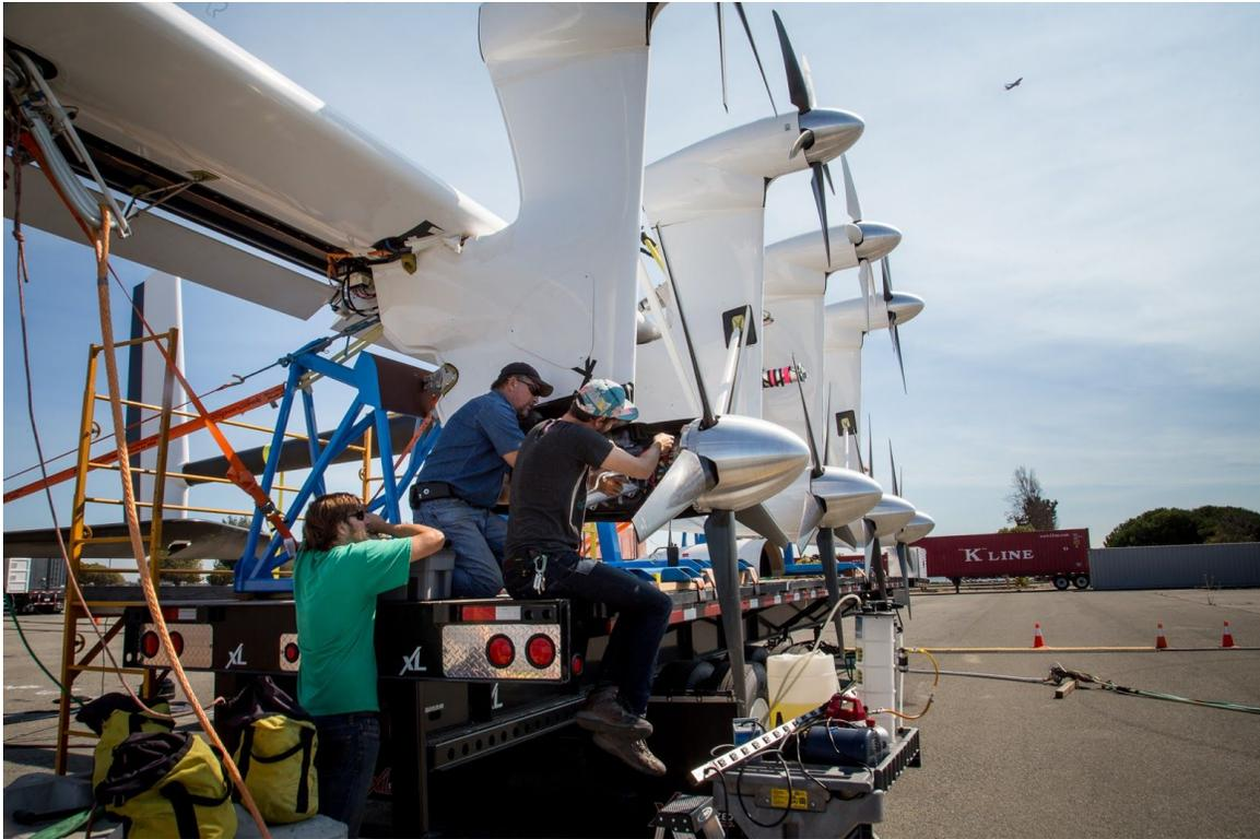
**Figure 15: Swapping a powertrain in the field required pumps to flush and refill the coolant.**
