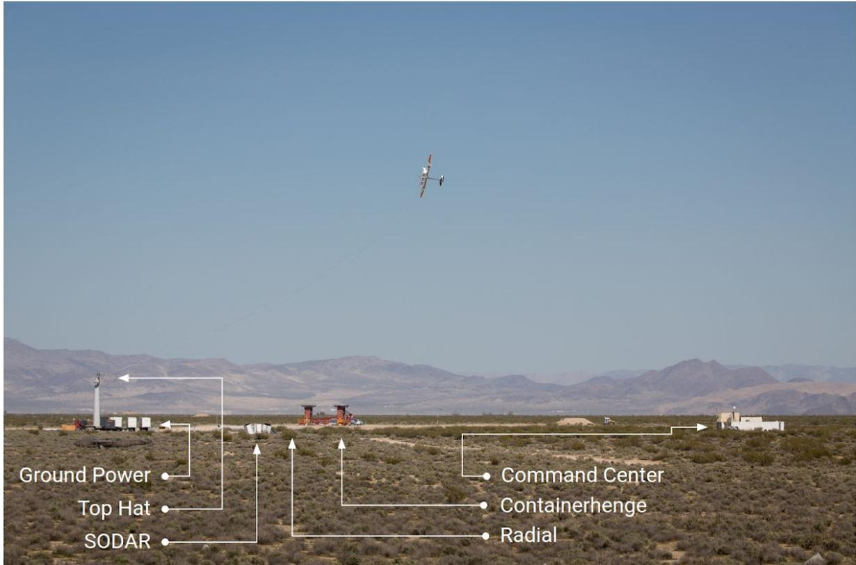
**Figure 4: China Lake Test Site. The kite is seen in crosswind flight, and the ground equipment visible from the ground includes (from left to right): the tower and Top Hat, three containers with the ground power inverters and switchgear, the SODAR wind profiler, Containerhenge further back along the cleared radial, and the command center on the far right.**
