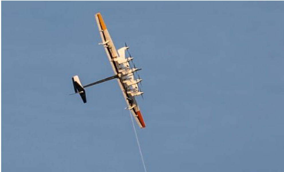
Fig. 1: The M600 energy kite has 8 turbines and a 25 m wingspan.
