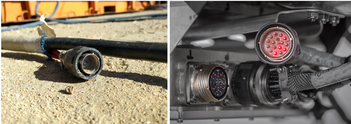
Fig. 8: Plastic fiber for high-density optical connections in harsh environments.
