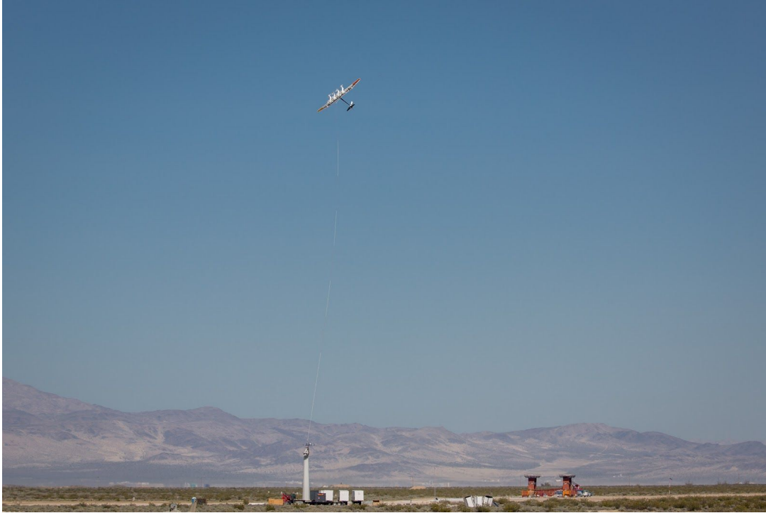
Makani's "M600" 600kW prototype operating in California, 2018.
