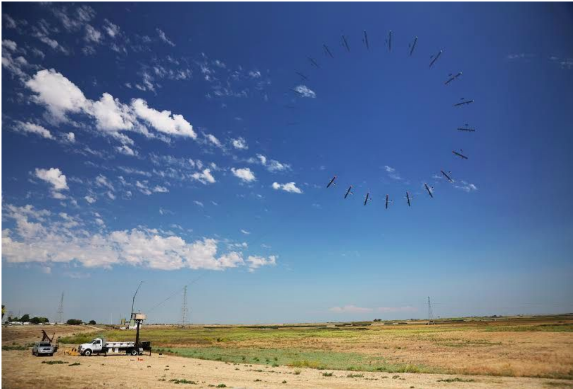
Layered photographs of the kite in flight around different points on the crosswind loop illustrate the flight path of Makani’s “Wing 7” 20kW prototype operating in California, 2013.
