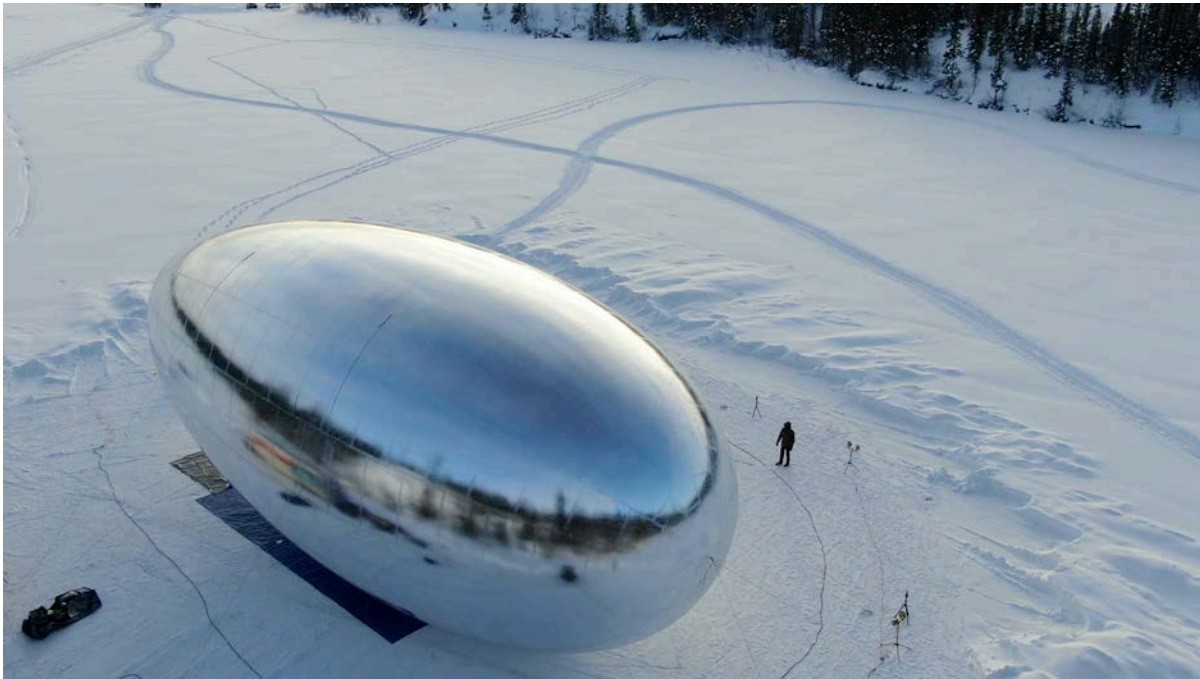
Figure 8-2 Jefferson fabric envelope testing. Taking advantage of -40°C weather in Yellowknife, Canada, to test fabric and envelope strength under pressure.
