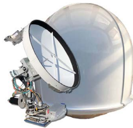
Figure 4-35 Loon Ground Station (left) and Radome (right) and two ground stations mounted on rapid deployment Conex.
