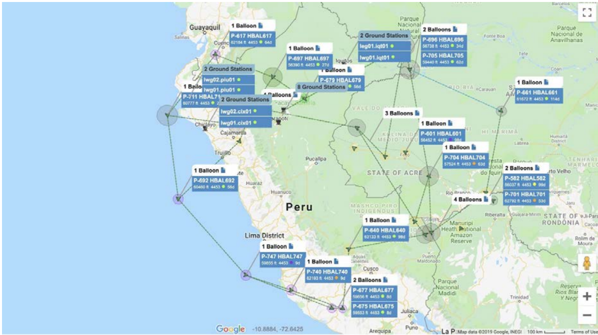
Figure 1-6 Loon fleet over Peru, Bolivia and Brazil. Loon fleet management system dashboard showing mesh backhaul network serving LTE users in Loreto region.
