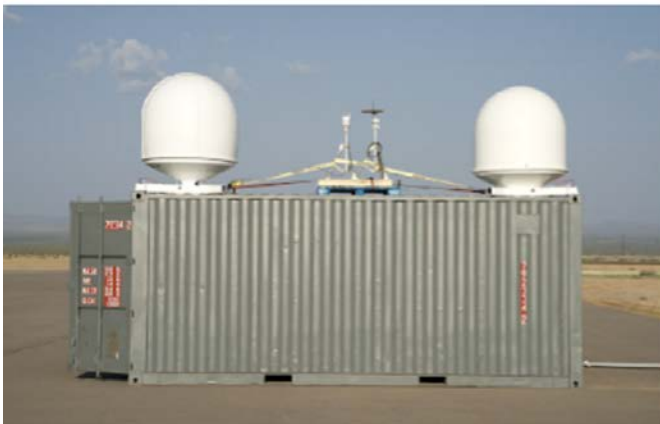
Figure 4-35 Loon Ground Station (left) and Radome (right) and two ground stations mounted on rapid deployment Conex.
