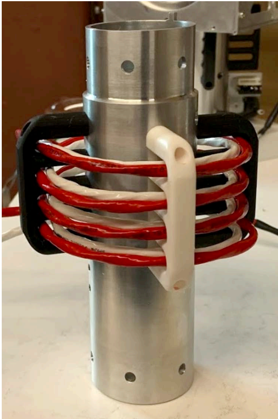
Figure 3-42 Pointing axis cable helix.
