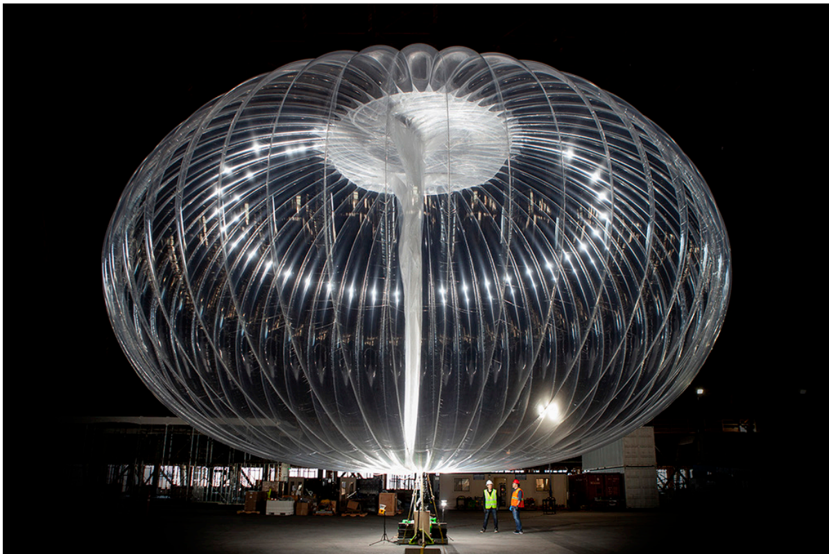
Figure 8-4 Loon's PE01 pumpkin balloon—starting point for Raptor balloon design.
