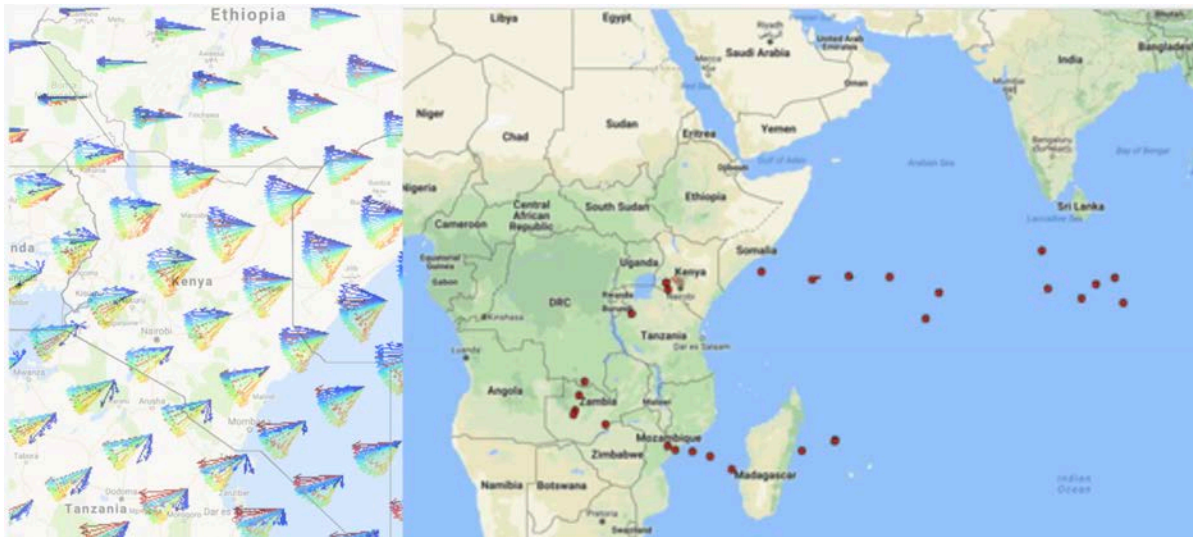
Figure 2-3 Wind cones and overprovisioning. Simulation of overprovisioned fleet serving southwest Kenya, with a 10,000 to 15,000 km return loop. On the left are the different wind directions found across the balloon’s altitude range showing that, across Kenya, vehicles will be consistently blown westward.
