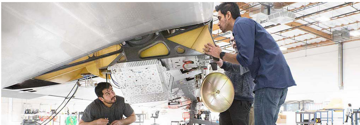
Figure 4-41 Loon and HAPSMobile. Loon team members finalizing integration of Loon payload into HAPSMobile Sunlider aircraft in late 2019.
