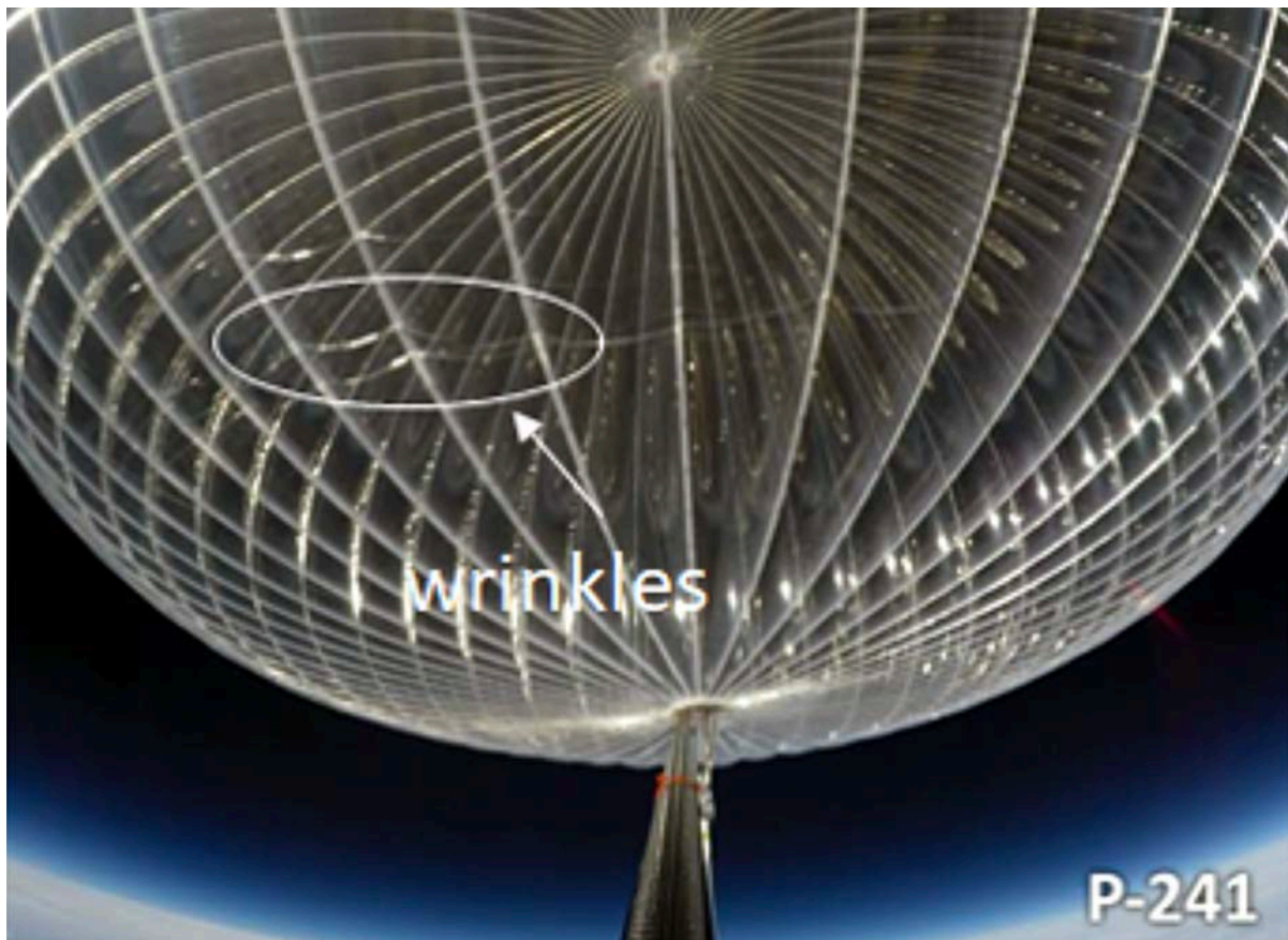
Figure 3-9 Envelope-only balloon in-flight. Gore wrinkles shown in the fully inflated state.
