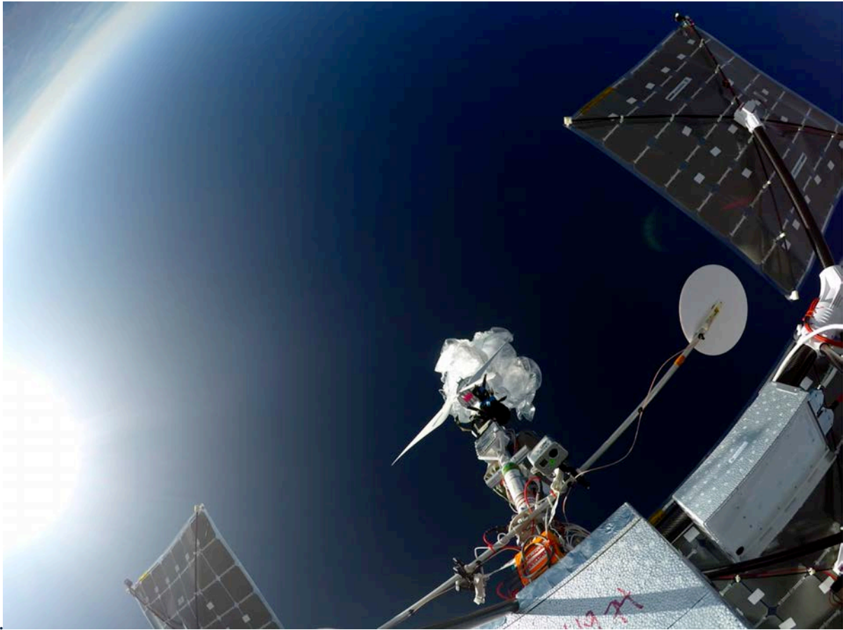
Figure 3-61 Special test flight showing the fully vented balloon in vertical train above the bus at upper altitudes.
