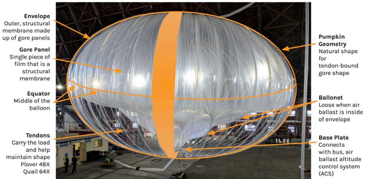
Figure 3-5 Inflated balloon and major components. Also note the size, relative to the people at the bottom left corner.
