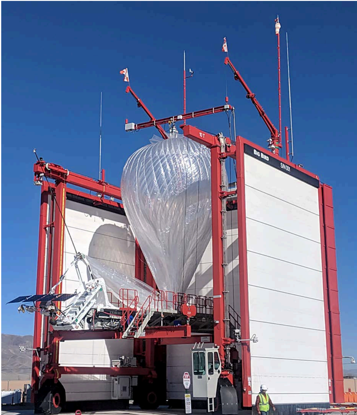
Figure 3-22 Balloon filled prior to launch.
