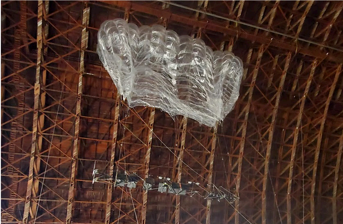
Figure 8-13 Bumpy Football and Alphadon bus with propulsion undergoing Soft Launch tethered testing.
