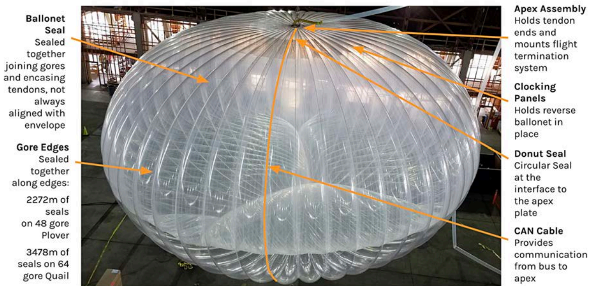
Figure 3-6 Inflated Plover balloon inside a hangar.
