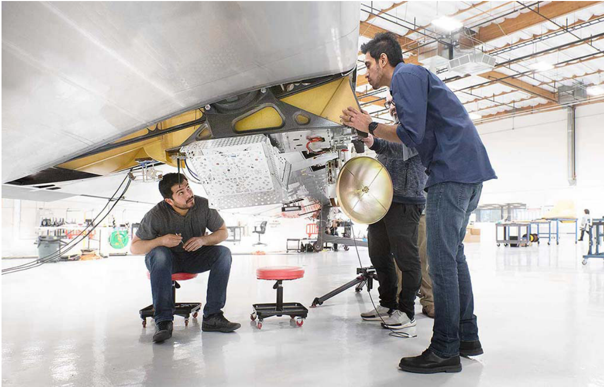
Figure 1-5 Loon on other aircraft. Fitting the Loon payload on a SunGlider aircraft.
