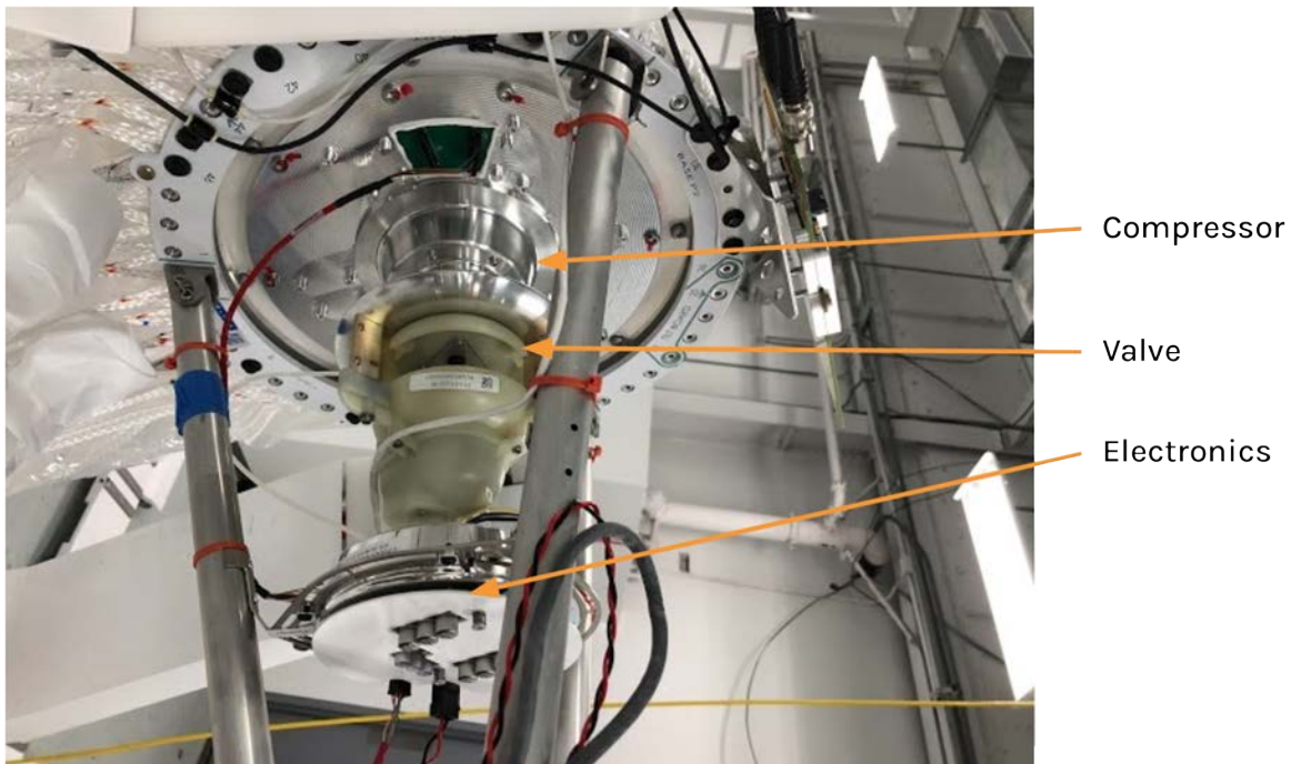
Figure 3-26 Major ACS components mounted for flight on the bottom assembly and campstool.
