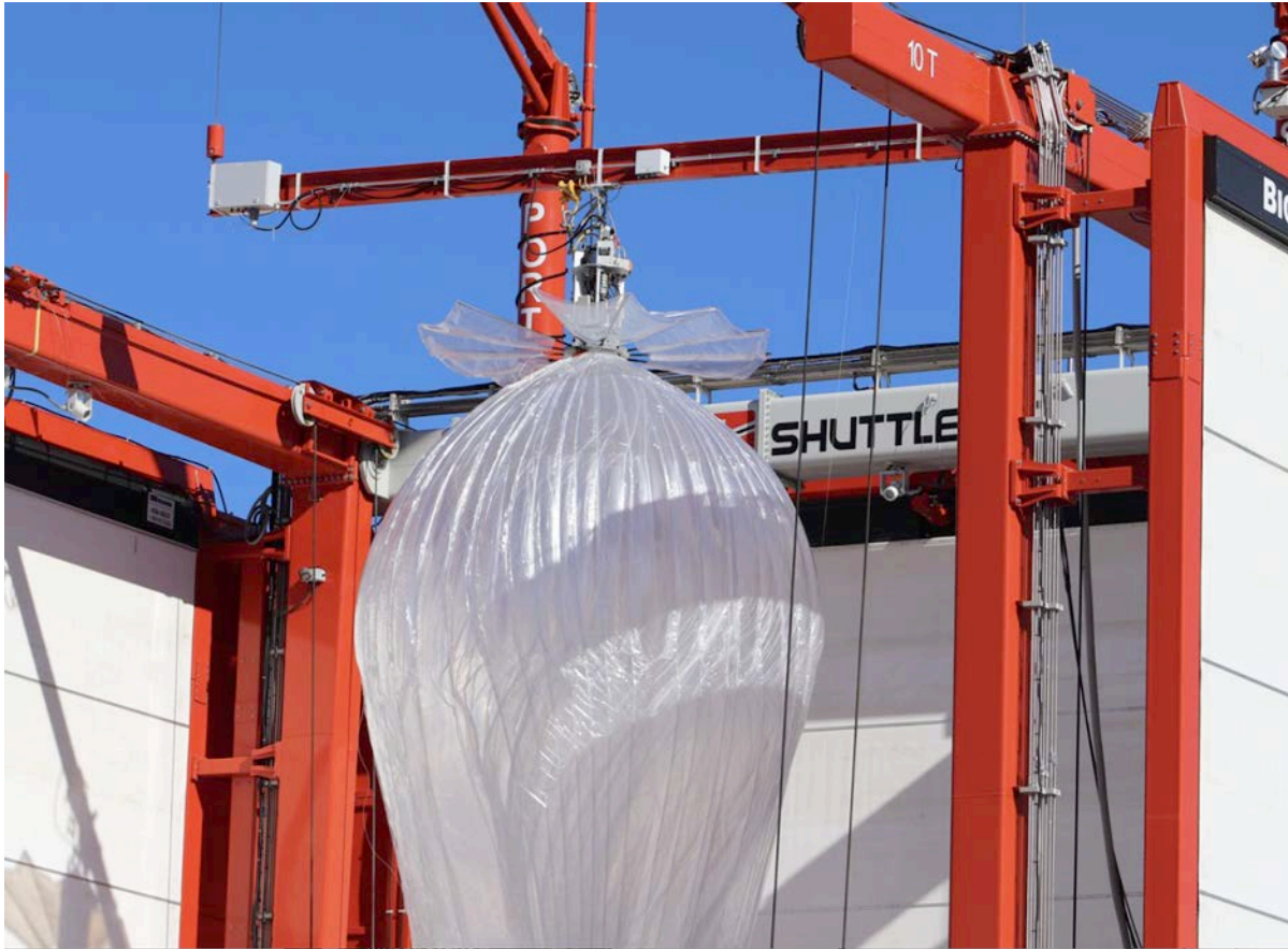
Figure 3-63 Drag disk prototype ready for a test flight.
