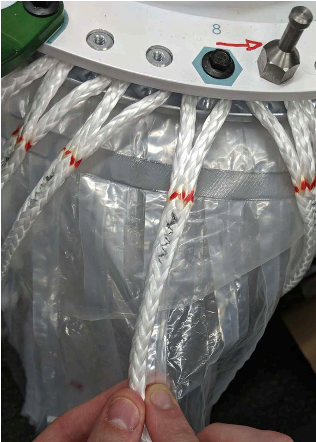
Figure 3-12 Braided DM20 tendon attached to the apex assembly load ring.
