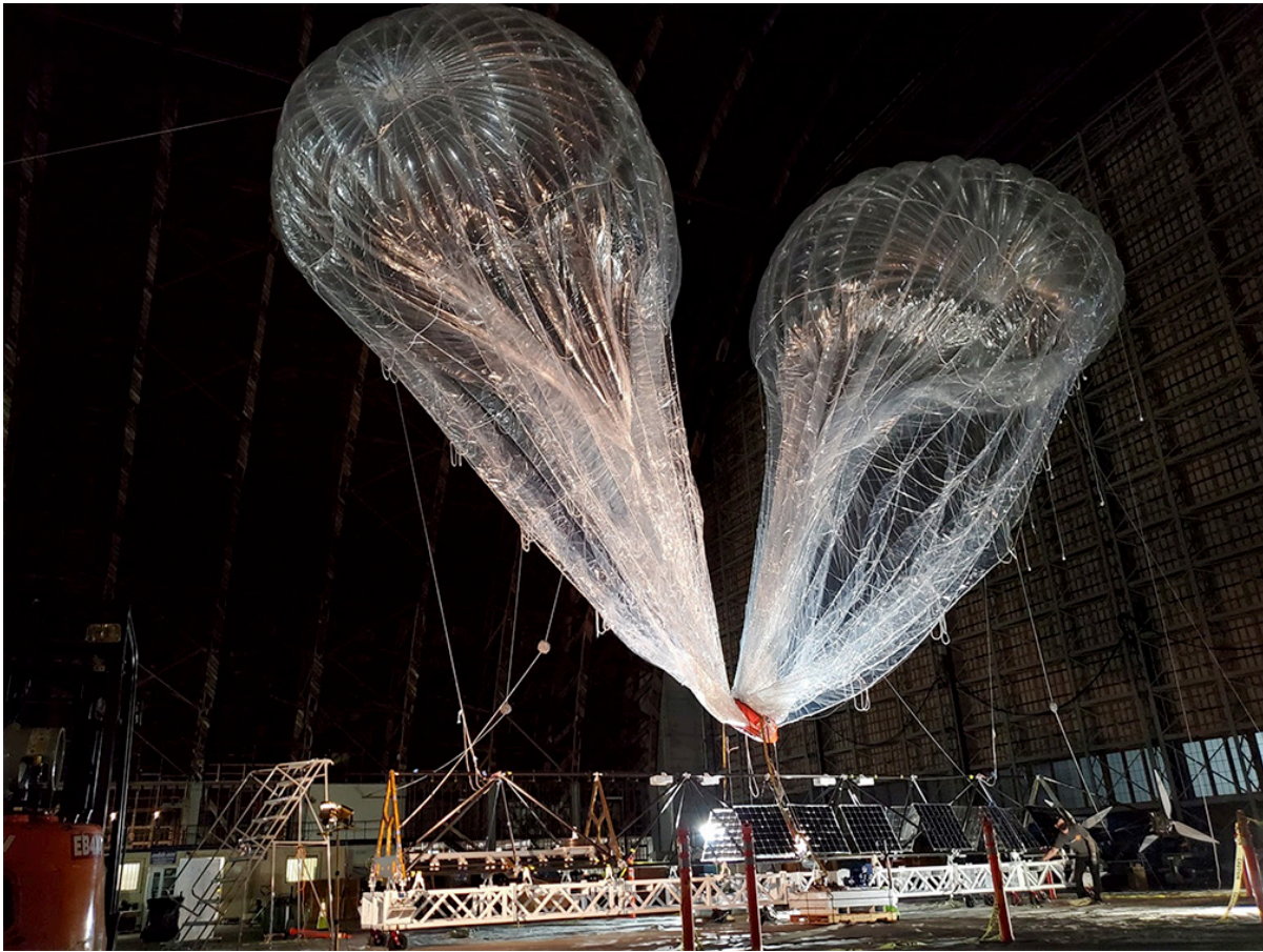
Figure 8-14 Vee Launch fill process as part of Soft Launch.
