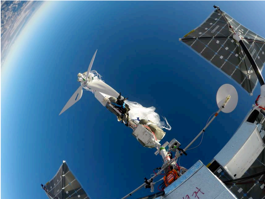
Figure 3-62 Special test flight showing momentary increase in balloon terminal velocity relative to the bus at lower altitude.
