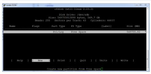
The cfdisk command provides a text user interface (TUI) for editing the partition table. The following list describes how to navigate through the interface:
